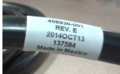
Figure 1 Incorrect power cord, falls within date range
