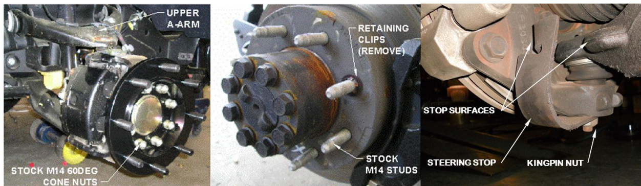
Figure 2 – Wheel Adapter Details
