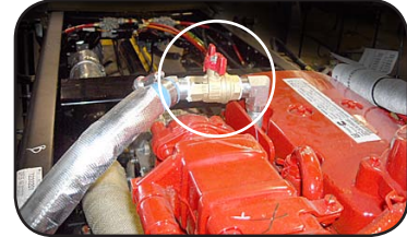
Forward Engine heater supply cutoff valve. Accessible from interior engine compartment hood.
