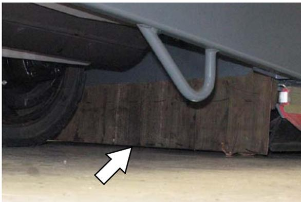
The skirts should be between 0 to 6 mm (0 to 0.25 in) from the floor when the scrub head is down.
