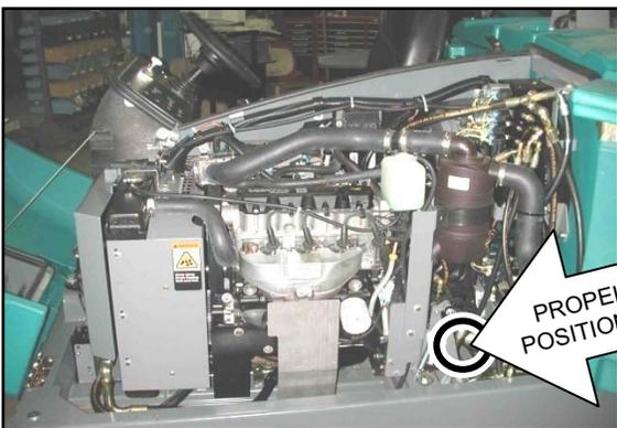
**i** See Forward Propel page for information on adjusting Propel Pedal Position Sensor
