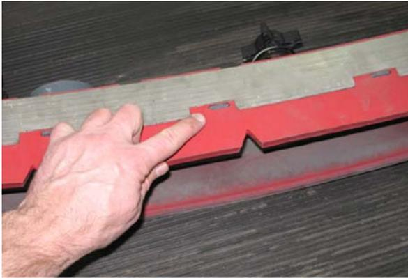
15. Tighten the front retaining band tension latch.
