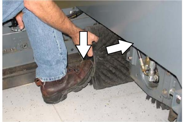
7. If rotating the existing brushes, only rotate front to rear. Do NOT rotate end-for-end.
