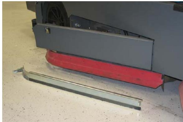
5. Remove the side squeegee blade. If the outer edge of the squeegee blade is not worn, rotate the squeegee blade with the blade from the other side of the machine. Discard the squeegee blade if both edges are worn.
