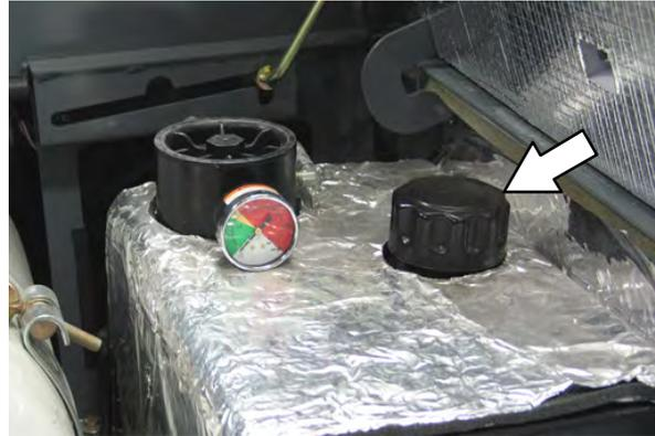
Replace the hydraulic fluid filter after every 1200 hours of operation or if the hydraulic reservoir gauge is in the yellow/red zone when the reservoir hydraulic fluid is approximately 32° C (90° F).
