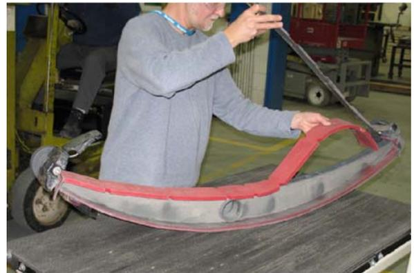
13. Install the new front squeegee blade or rotate the existing blade to the new edge. Be sure the holes in the squeegee blade are hooked onto the tabs.
