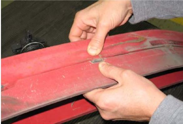
9. Reinstall the rear retaining band aligning the tabs with the holes.
