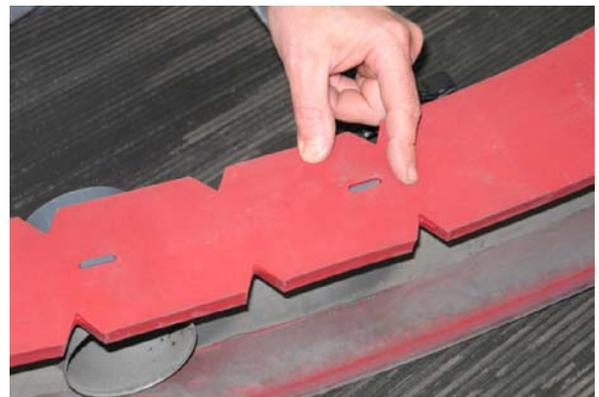
14. Reinstall the front retaining band aligning the tabs with the notches.
