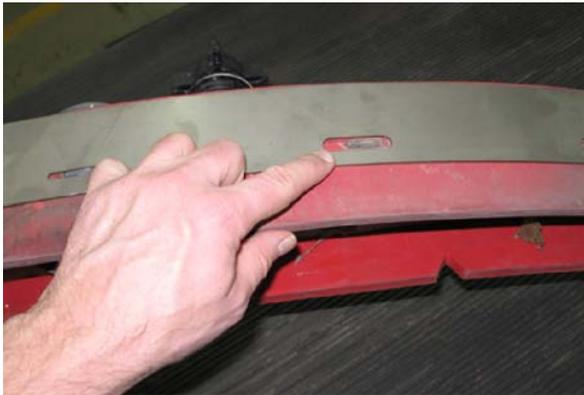
10. Tighten the rear retaining band tension latch.
