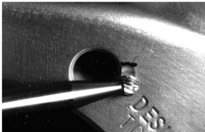
Figure 6. Crack Removal Using a Grinding Burr
