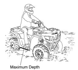
NOTICE: Major engine damage can result if the vehicle is not thoroughly inspected after operation in water. Perform the services outlined in the maintenance chart. See page 60. The following areas need special attention: engine oil, transmission oil, front and rear gearcase oil, and all grease fittings.
