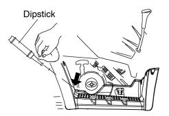
7. Remove the dipstick and check the oil level. Add oil as needed. Maintain the oil level in the safe range. Do not overfill.
