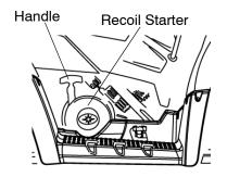
**Tip:** The rope will be harder to pull when the engine is on a compression stroke. When a compression stroke is found, continue pulling the rope just until the engine rolls past the stroke, then stop pulling immediately.
