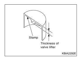
Thickness of a new valve lifter can be identified by stamp marks on the reverse side (inside the cylinder).
