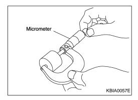
3. Measure the center thickness of the removed valve lifters with a micrometer.
