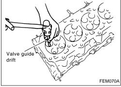
2. Using valve guide drift (multi-purpose tool: for 7.0 mm dia.), tap valve guides out from the combustion chamber side.
