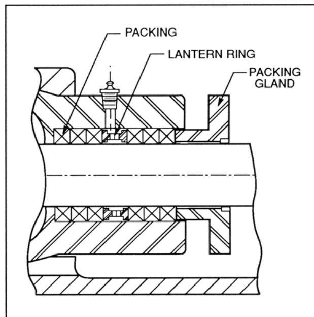
**Figure 4-1. Cross Section of Packing Retainer**
