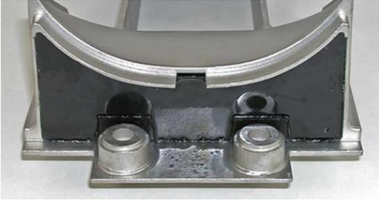
Test fit intake grate to ensure it seats properly in hull. Variances in materials (hull, transom plate, pump seal kit) may require the Pump Seal Kit be relieved to allow intake grate to be installed properly.
