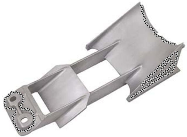
Install intake grate and secure with stock bolts. **NOTE: Apply blue Loc-tite to bolts. Torque to 29 lbf•in / 40 N•m.**
