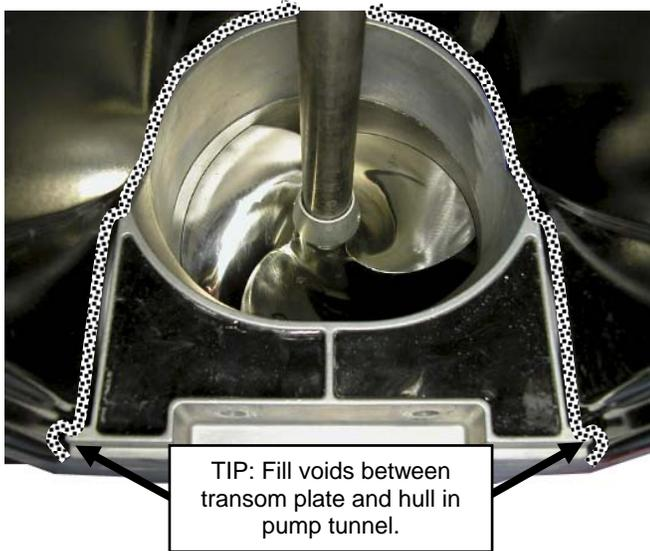
Apply a generous amount of 'below waterline' silicone sealant to all exposed surfaces of pump seal kit inserts in intake grate.
