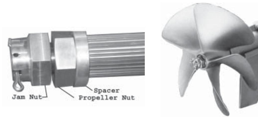
Figure 24. Propeller Retaining Parts (left), and Propeller Installed (right)
