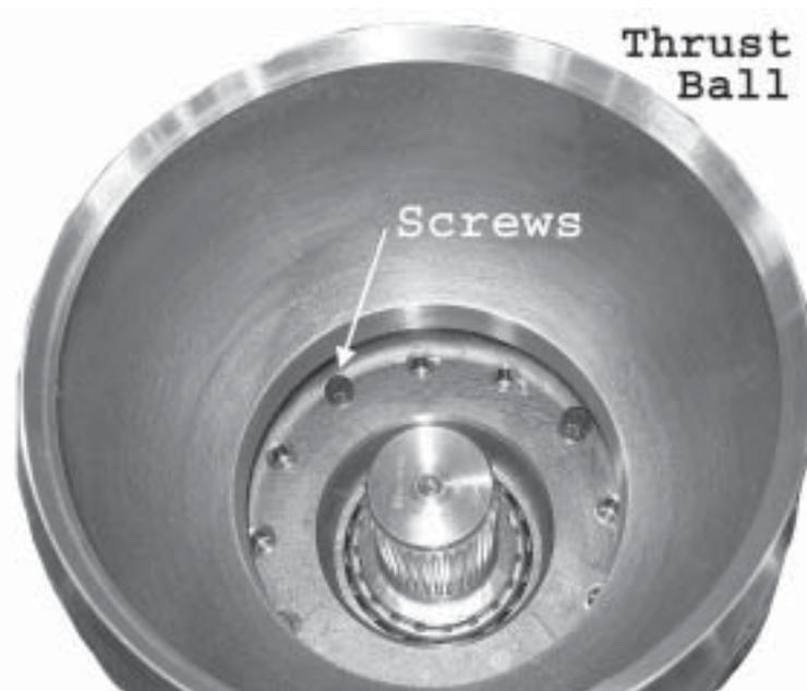
**Figure 37. Rotate Thrust Tube Assembly so Ball is Up, Remove 12-point Capscrews**
