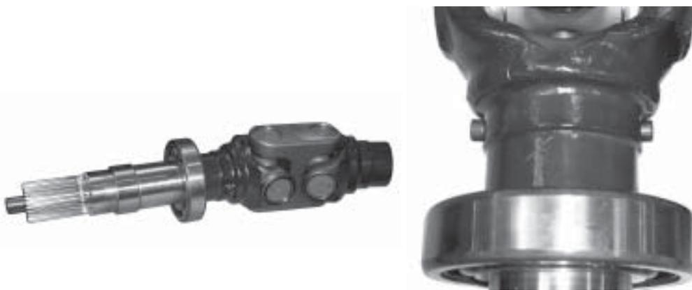
**Figure 72. Lower U-joint onto Spline (left), Install Collars (right)**
