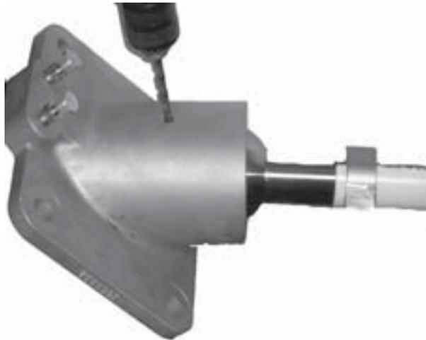
**Figure 99. Drill 1/8" into the retainer threads.**
