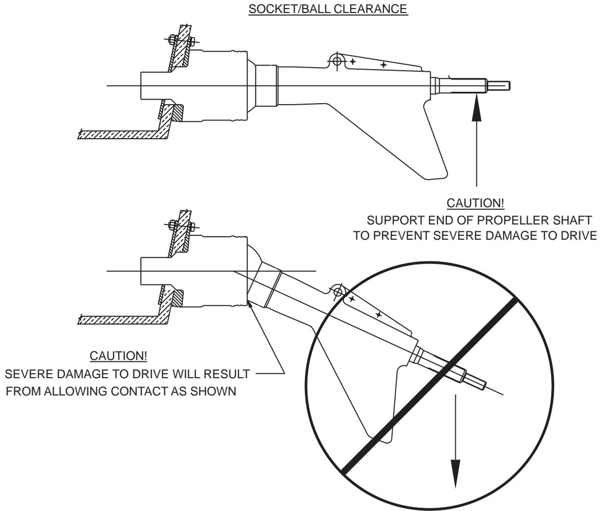
**Figure 32. Protect Ball from Damage**
