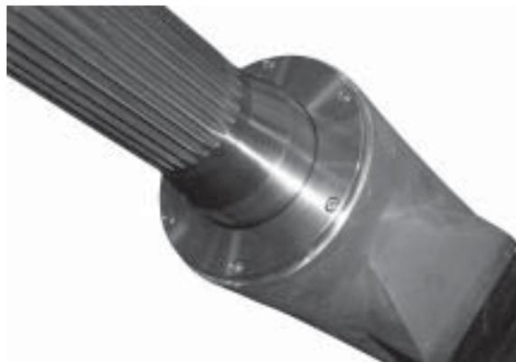
**Figure 70. Install Seal Carrier**
