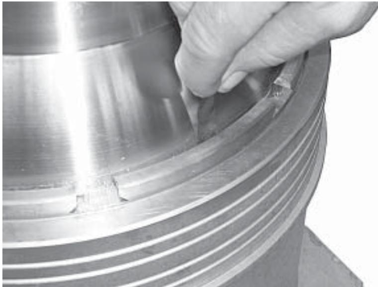
**Figure 82. Measuring the Gap Between Thrust Ball and Aft Retainer**
