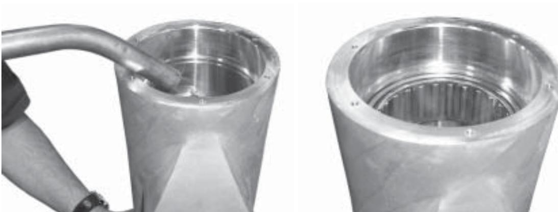
**Figure 55. Installing Aft Thrust Tube Bearing**
