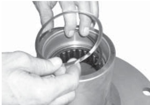
**Figure 75. Installing Retaining Ring**
