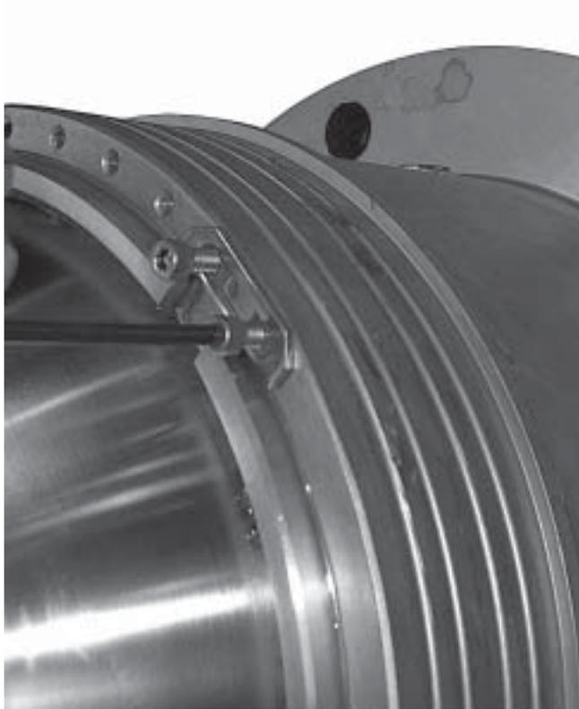
**Figure 35. Aft Retainer Ring Lock Clip in the Notch Locking Tab**
