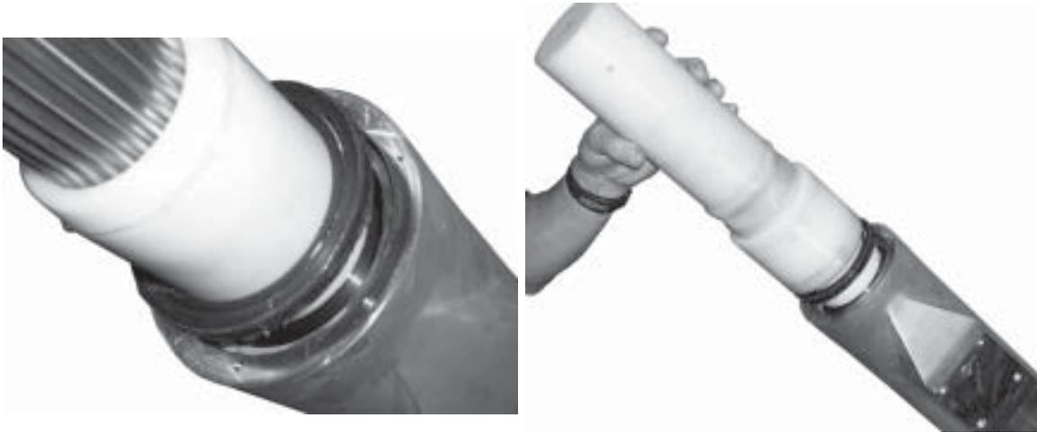
**Figure 69. Installing Outer Seals (left), Using Seal Driver (right)**
