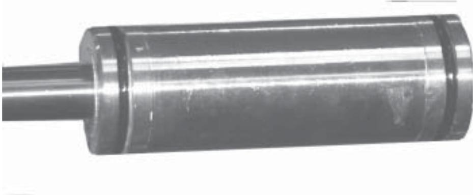
**Figure 95. Slide the piston on to the rod.**
