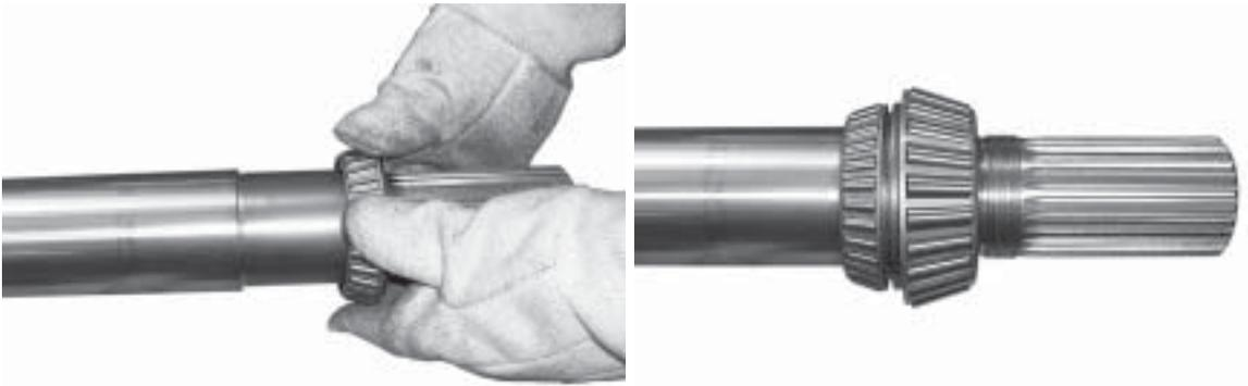
Figure 50. Install Tapered Roller Bearings
