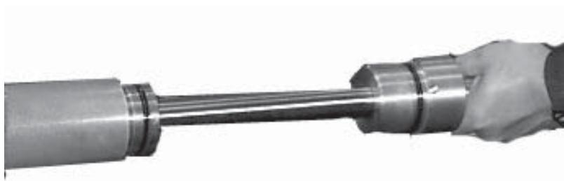
**Figure 97. Insert the piston rod assembly into the tube.**
