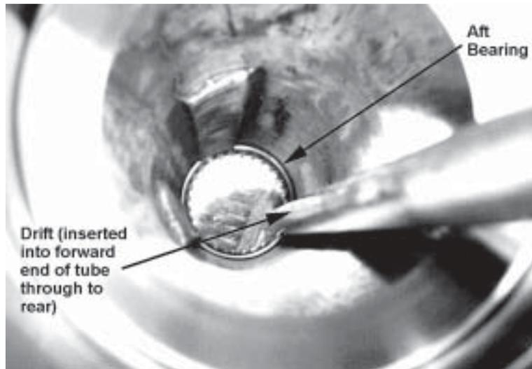
**Figure 40. Inserting drift into thrust tube to remove aft bearing**
