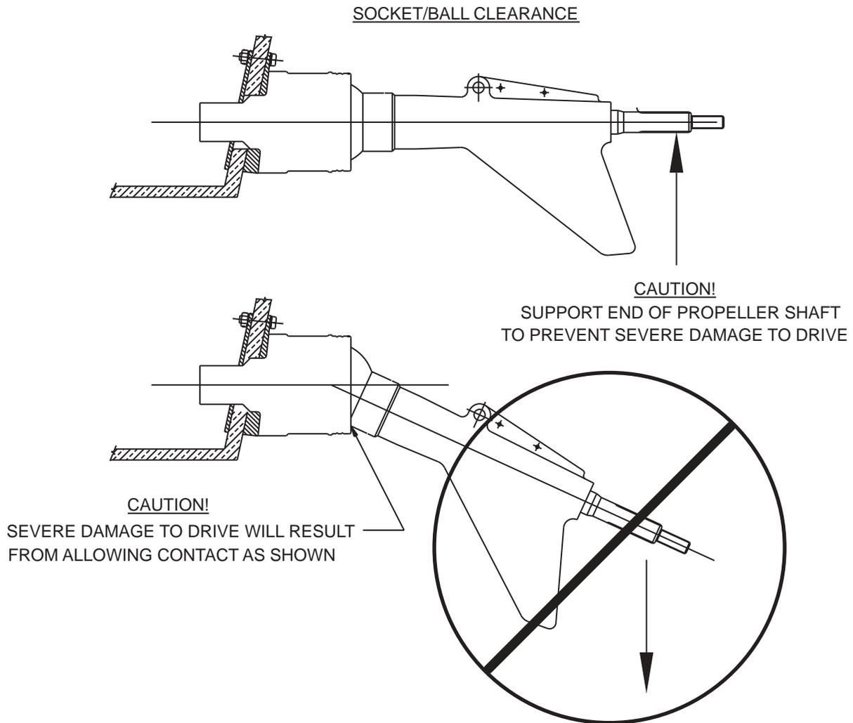
**Figure 25. Protect Ball from Damage**
