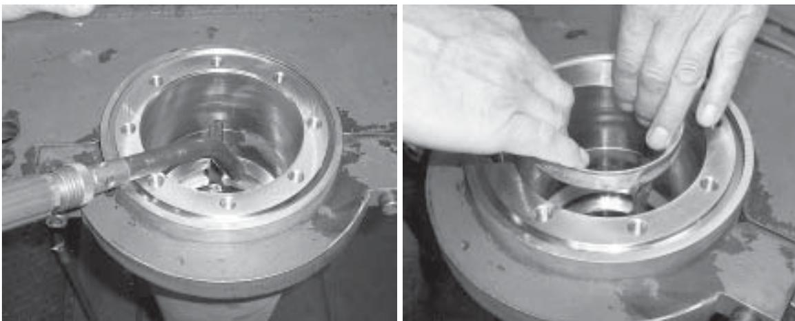
**Figure 57. Installing First Bearing Cup**
