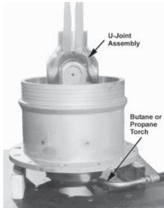
**Figure 45. Heating Housing to Remove U-Joint Assembly**
