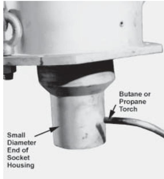
**Figure 46. Heating Housing to Remove Roller Bearing from Small Diameter End**
