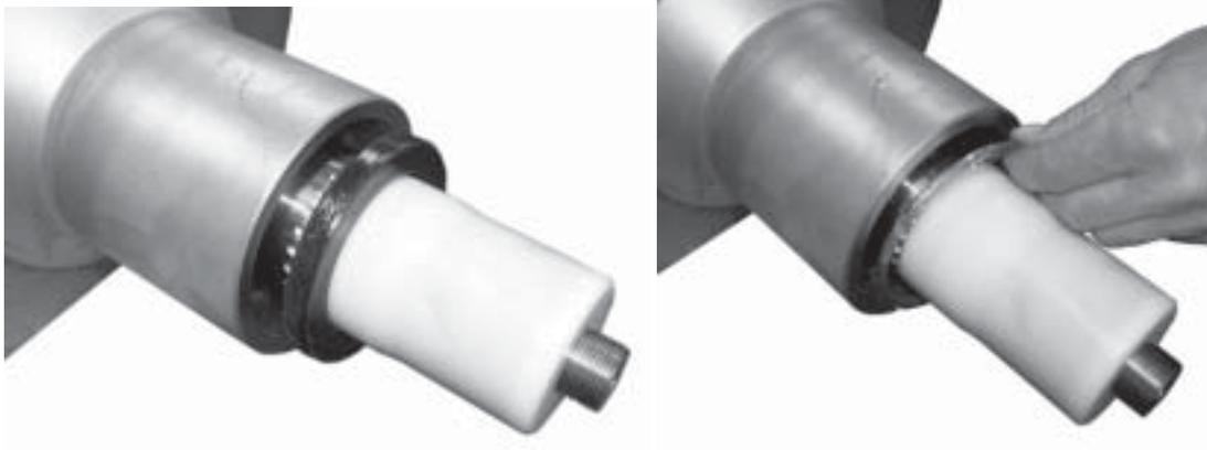
**Figure 83. Installing Front Oil Seals and Spacer**
