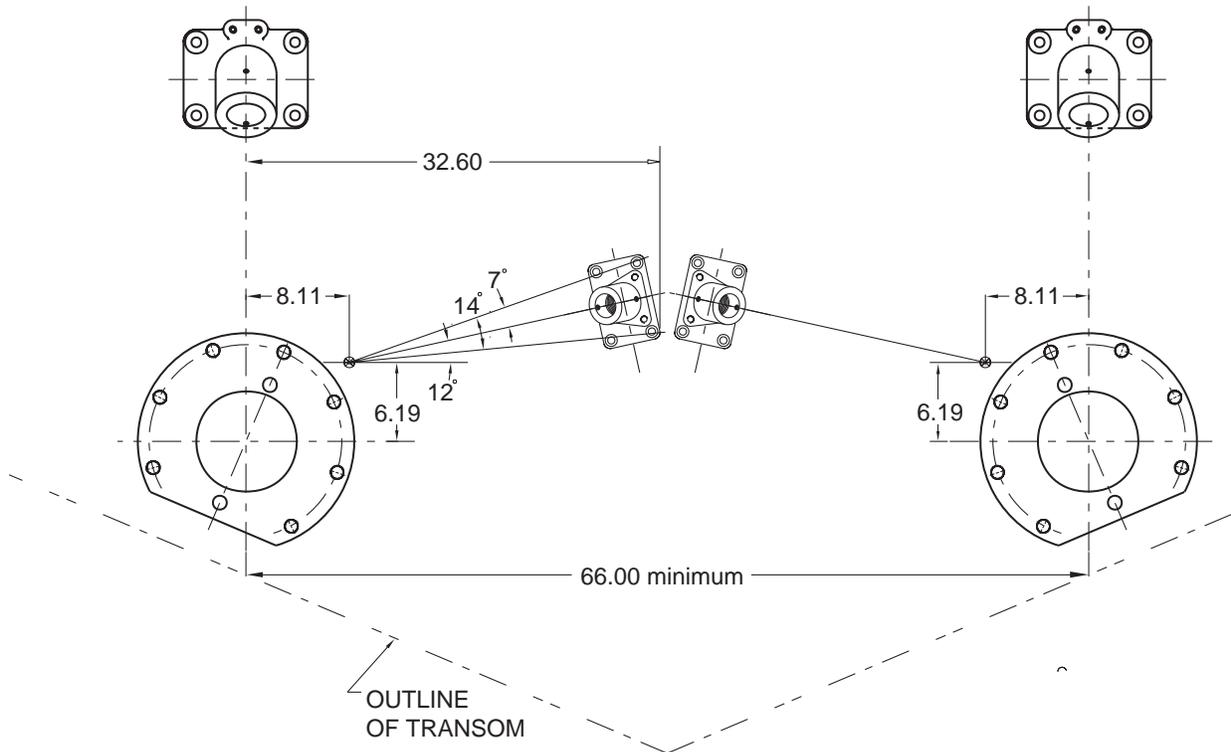
**Figure 15. Transom with Optional Inboard Steering**
