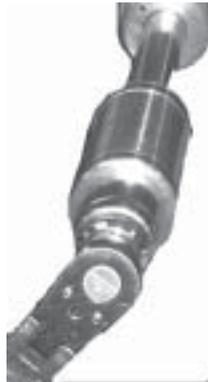
**Figure 96. Tighten the flexloc nut.**
