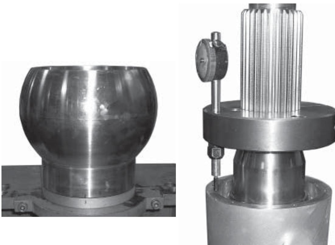
**Figure 61. Lower Ball, Secure with Four Capscrews (left), and Turn Over and Install Dial Indicator T-21549-11 (right)**
