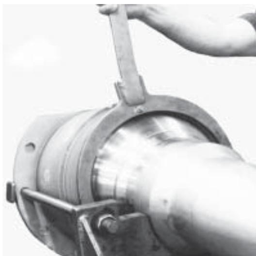
**Figure 81. Tightening the Aft Retainer using Special Wrench**
