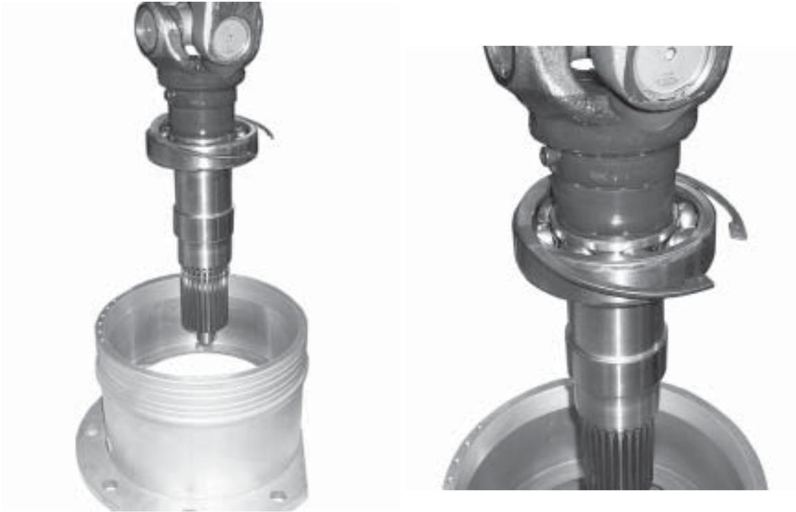
**Figure 76. Installing Input Shaft and U-Joint into Socket**
