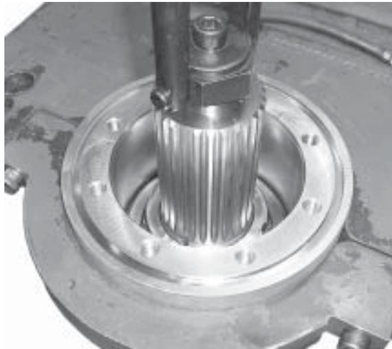
Figure 38. Remove propeller shaft
