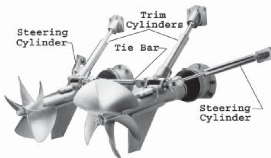
**Figure 26. Rear View of Dual Installation Showing Cylinders and Tie Bar**
