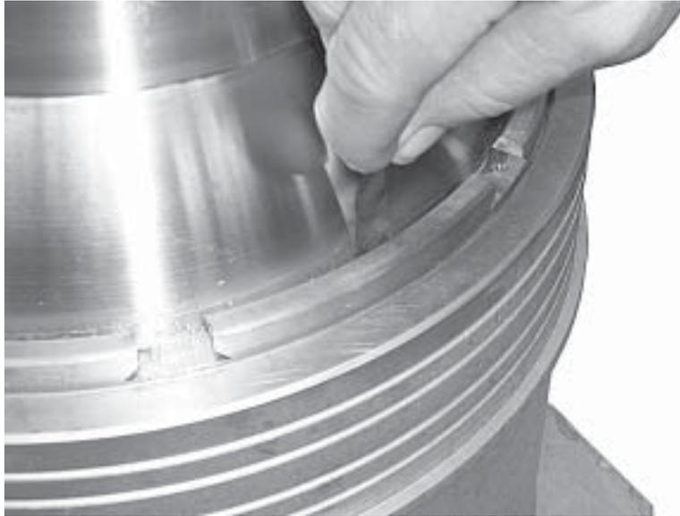
**Figure 34. Measuring the Gap Between Thrust Ball and Aft Retainer**
