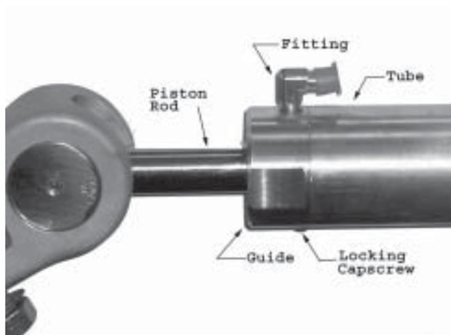
**Figure 90. Steering Cylinder.**
