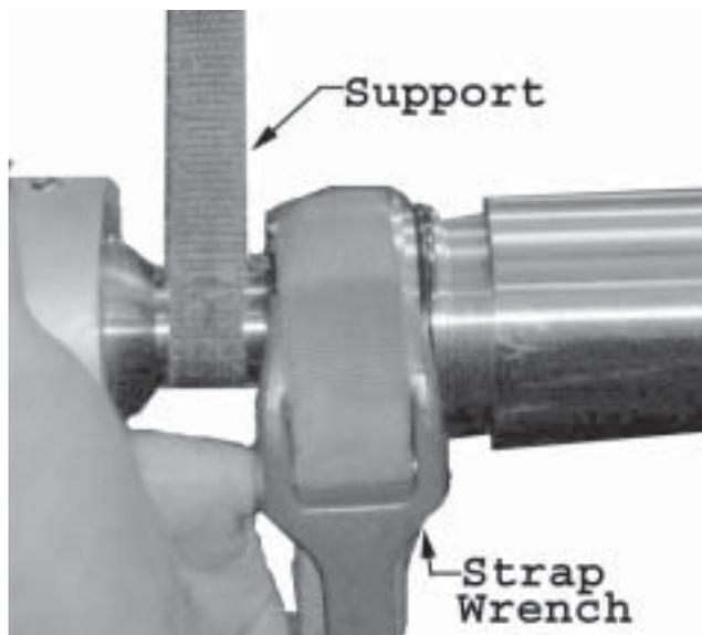
**Figure 107. Tighten the guide.**
