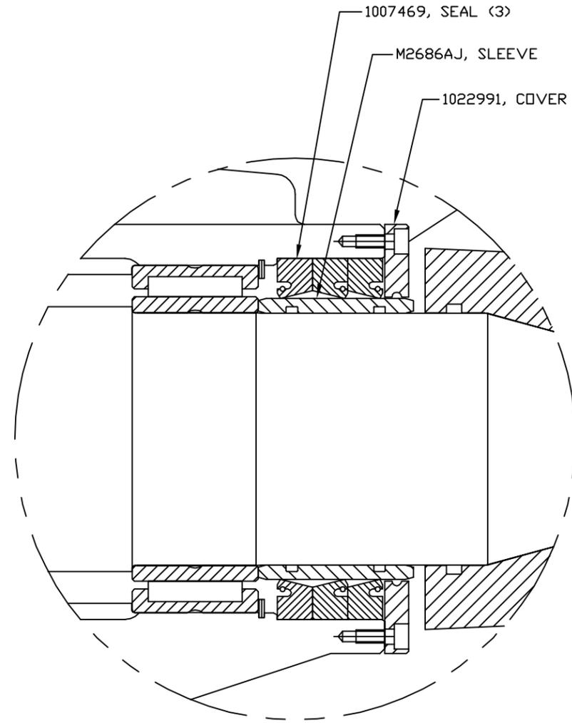
TRIPLE AFT SEAL ARRANGEMENT
