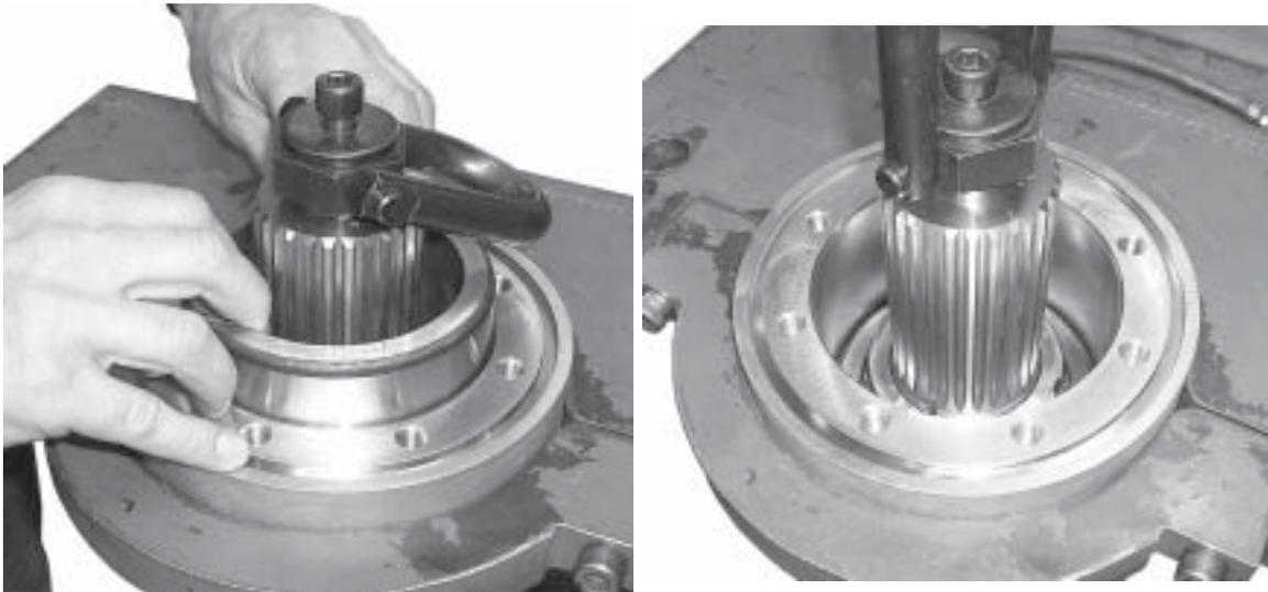
**Figure 60. Install the Chilled Front Bearing Cup (left), and Raise the Shaft to Ensure End Play (right)**
