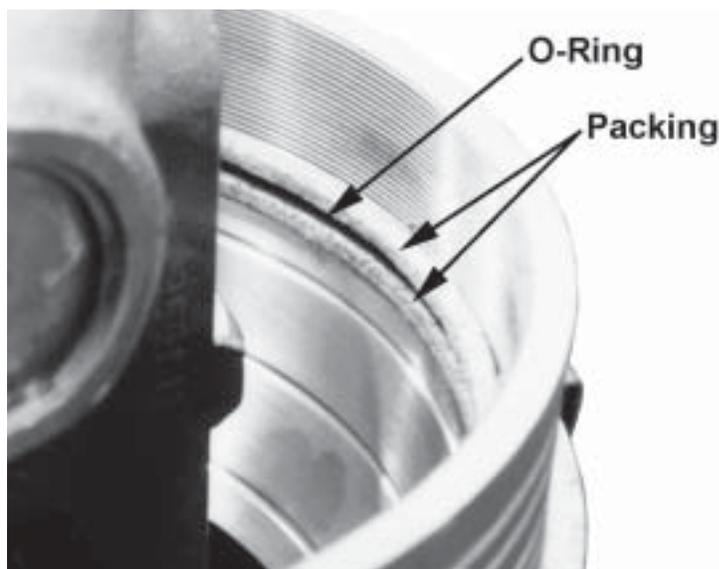
**Figure 79. Replacement of Thrust Socket Packing and O-Ring**
