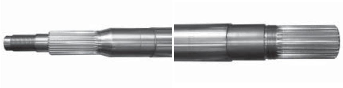
Figure 49. Propeller Shaft - Propeller End (left), Forward End (right)
