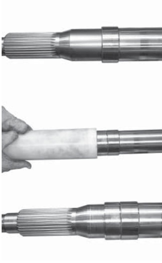
**Figure 54. Sliding the Heated Bearing Race on the Shaft**
