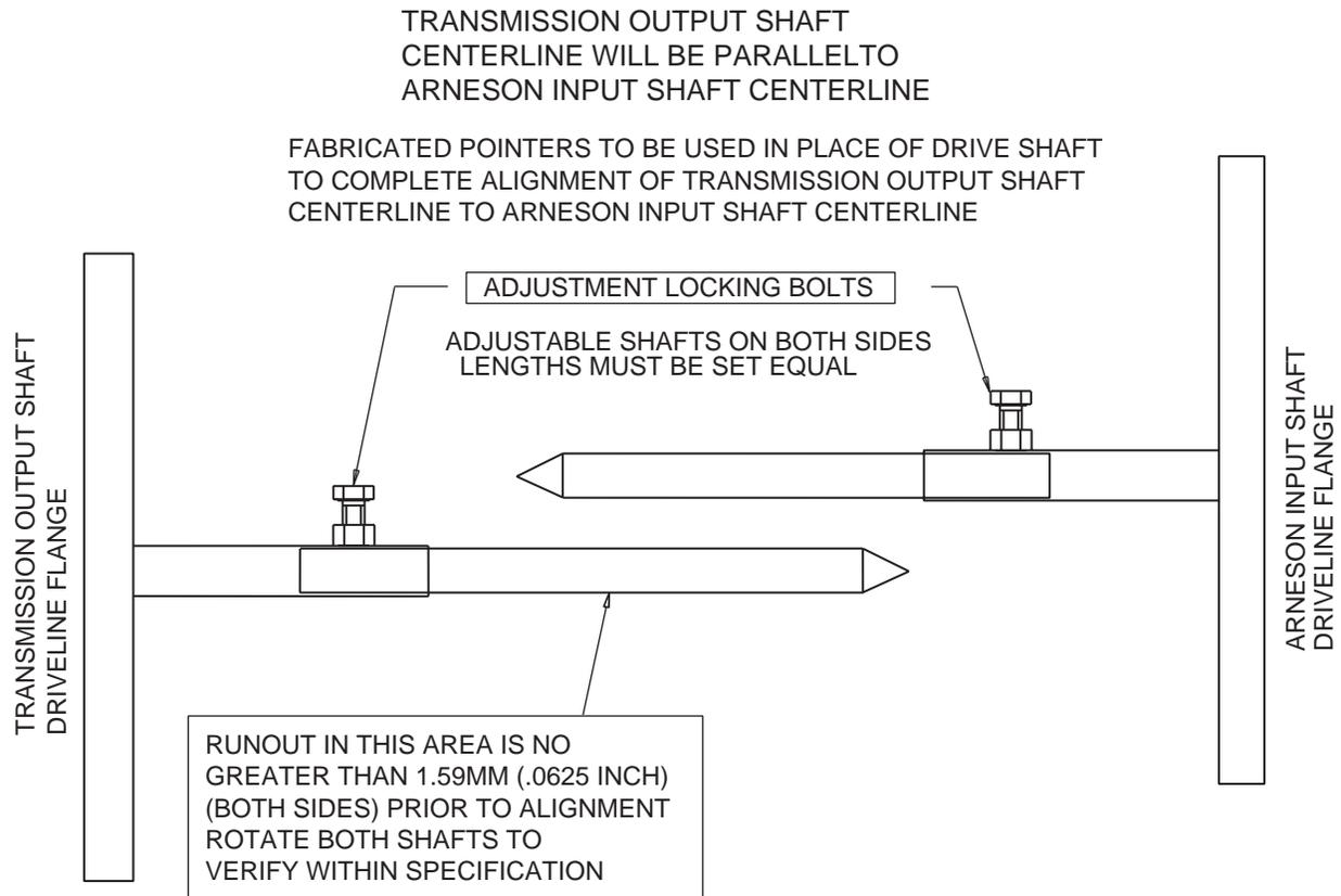
**Figure 19. Remote or Island Mounted Alignment Tool, Shafts Parallel**
