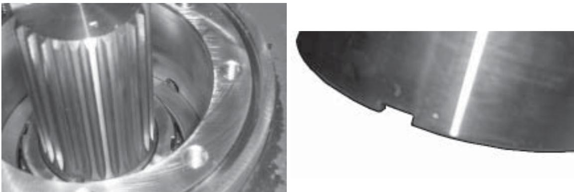
**Figure 63. Case Slot (left), Thrust Ball Slot (right)**
