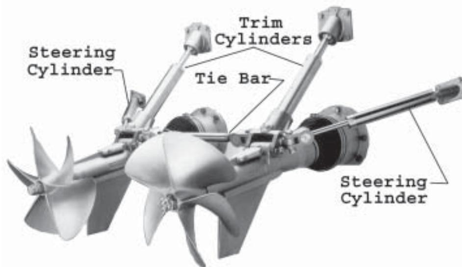
Figure 31. Rear View of Dual Installation Showing Cylinders and Tie Bar
