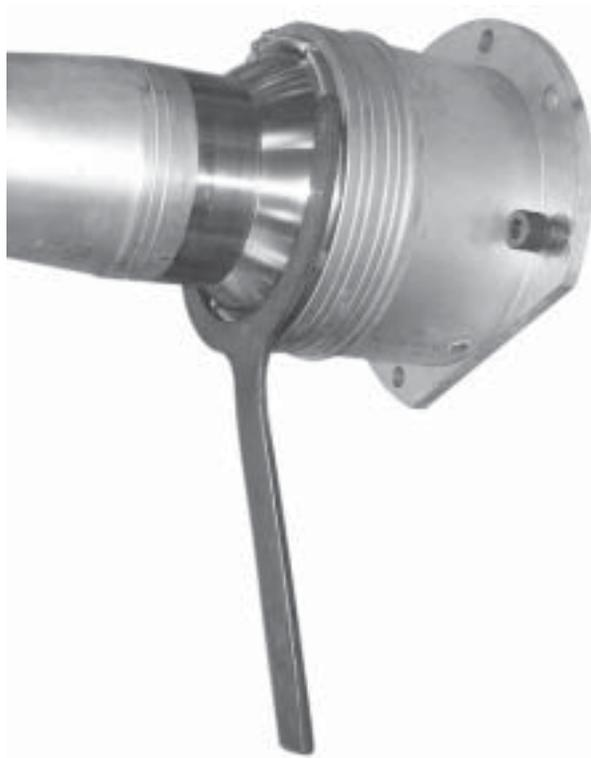
**Figure 29. Unscrewing threaded Aft Retainer**
