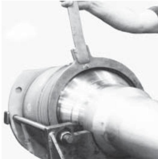
**Figure 36. Removing the Aft Retainer using Special Wrench**
