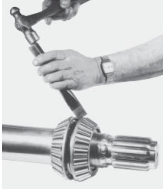
**Figure 42. Breaking Bearing Cage With a Chisel**
