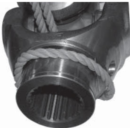
**Figure 80. Support U-Joint During Installation of Thrust Tube into Thrust Socket**
