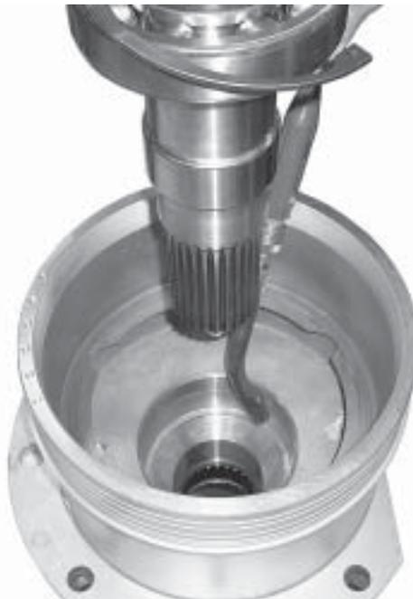
Figure 77. Installing Input Shaft and U-Joint into Socket
