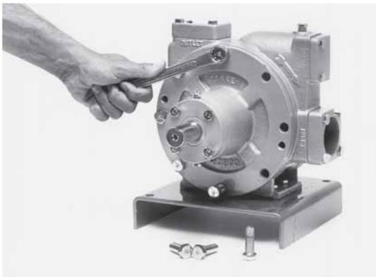
Loosen the head bolts and remove one head with the bearing cap attached, while holding in on the shaft.
