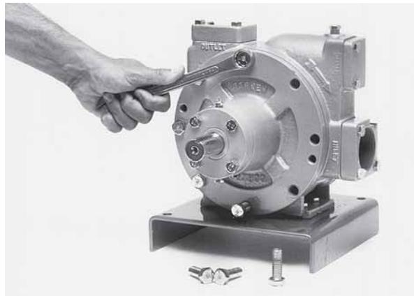
Torque the head bolts in a crossing pattern. There is no need to disassemble or re-shim the bearing caps. Repeat all of the above steps when replacing the seal assembly on the opposite side.
