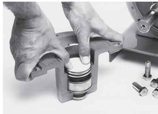
**NOTE:** *The above photo is of a cutaway for better details.* Turn the head over and install the new grease seal face down by pressing into the bore behind the main bearing. This can best be accomplished using the old seal seat with the O-ring removed. Apply a generous amount of light oil to the new seal seat. Using the protective disc, gently press seal into place.
