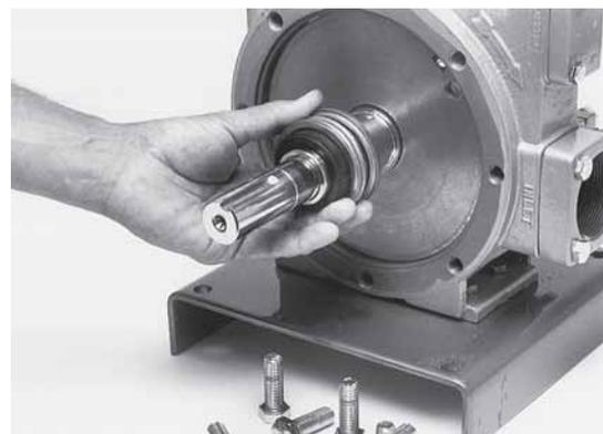
Remove the old seal assembly from the pump shaft while pressing against the sideplate. This will allow the seal retainer assembly to be removed without pulling the rotor-shaft out of the pump.
