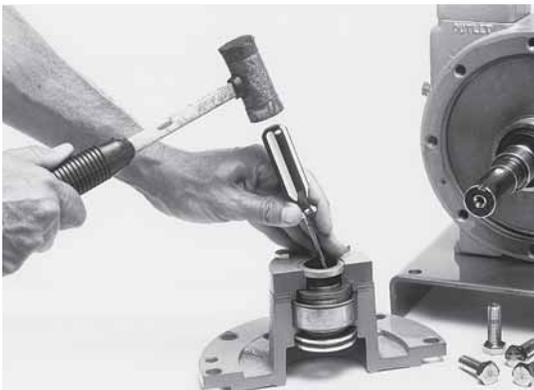
**NOTE:** *The above photo is of a cutaway for better details.* Remove the head O-ring and place head on the workbench as shown. Lightly tap the seal out of the head with a long screwdriver by reaching through the bearing cap opening. Inspect the inner lip seal and remove, if necessary, using same process.
