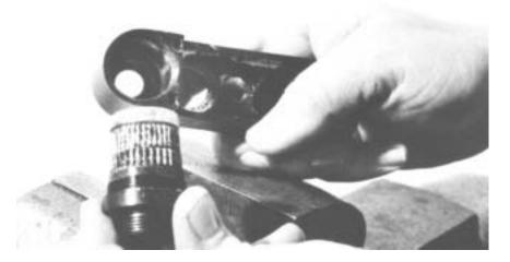
17. Remove nose adapter (left hand threads), spindle drive gear 622950, spindle feed gear and spindle feed gear bearing 617168.
