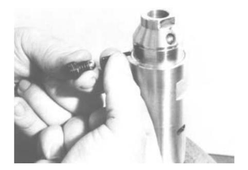
30. Unscrew spring retainer 613060 and remove spring 613058, ball 844077 and push rod 613264, for inspection.
