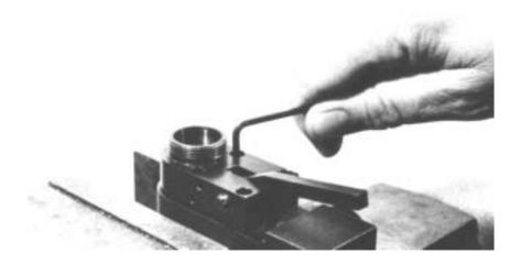
6. Remove four 7/64" socket head cap screws 863337 and lift off retract body 624094.
