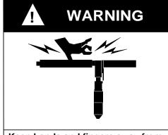
Keep hands and fingers away from slot in spindle guard and nose piece when handling or operating tool.
