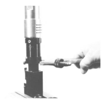
3. Clamp drill head in soft jawed vise in a vertical position and remove drill head and drill head adapter 613544 (both left hand threads).
