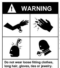
Follow good machine shop practices. Rotating shafts and moving components entangle and entrap, and may result in serious injuries. Never wear long hair, loose-fitting clothes, gloves, ties, or jewelry when working with or near a drill of any type.
