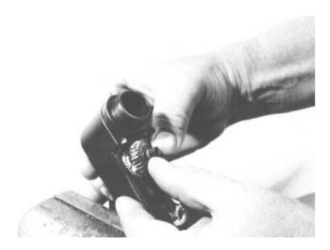
16. Press differential drive gear 622949 and differential feed gear together and slip out of housing 622986.
