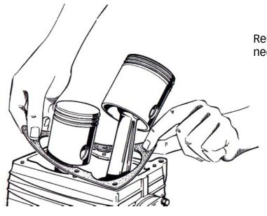
Replace cylinder gasket if necessary.
