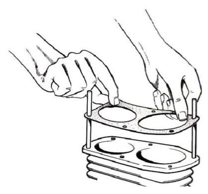
Guide pins may be used to fit gaskets and valve plates.
