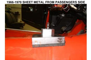
3. Complete by permanently attaching new metal by welding or other secure method. Use a seam sealer such as 3M Fast 'n Firm or equivalent between new and old metal. Paint both sides for corrosion protection. If large gaps exist between old and new metal, urethane foam can be used as a filling agent, then trimmed and painted after drying.
