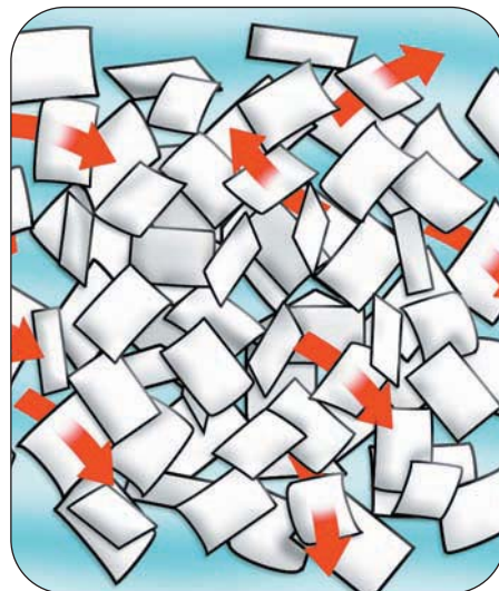
TIGHTLY PACKED: Chemicals cannot penetrate the entire load as quickly in a competitive tunnel.
