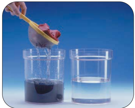
You can see the effect of total top transfer vs. other methods by using buckets of water to simulate different compartments. A Milnor loading scoop lifts the goods, drains them, and deposits them into cleaner water.
