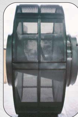
Water flows easily through Milnor's perforated cylinder.
