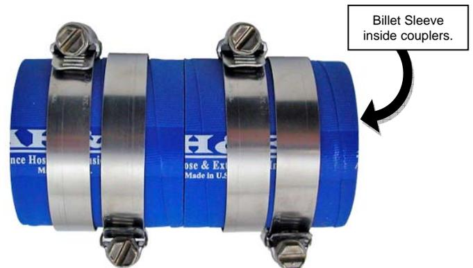
With one hand suspend assembly in hull between bulkhead and pump tunnel. Use freehand to slide couplers out onto flanges on hull.
