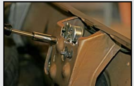
Figure 1B: Mounting the new electric trunk latch on a 1967-68 Mustang.
