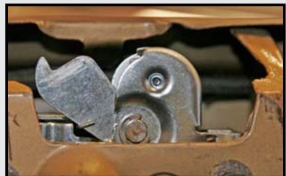
Figure 3A: Note the clearance on the trunk latch when checking the installation.
