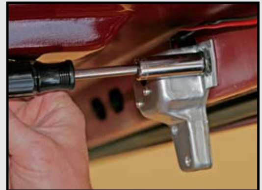
Figure 1A: Mounting the new electric trunk latch on a 1965-66 Mustang.
