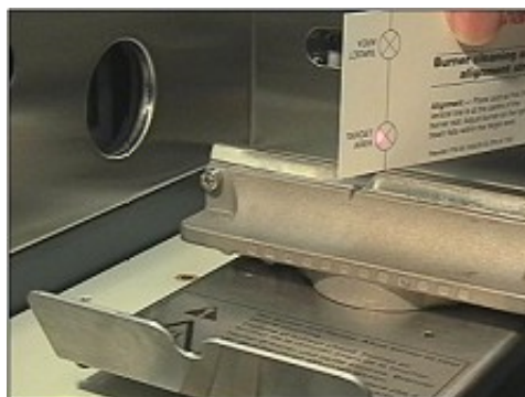
Figure 22. Aligning the burner
