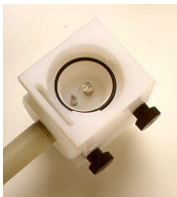
Figure 9. O-ring in place in the nebulizer block
