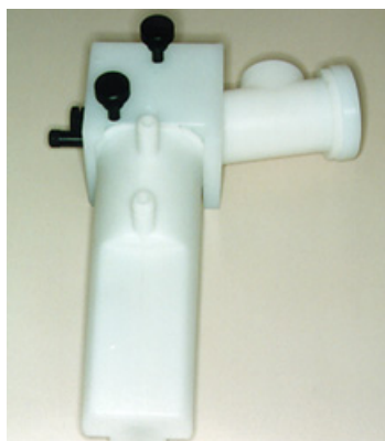
Figure 11. Complete nebulizer/spraychamber assembly
