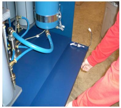
**Grasp tray** by handles. Carefully slide out for service. Switch stays in tray.
