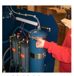
After fluid is dispensed through the output hose, shut down the system and check for leaks.
