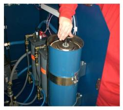
Loosen and remove the V-band Clamp at the top of the canister and remove the lid.
