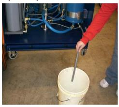
Locate the absorber drain hose. (It is folded over and tie-wrapped) Cut the tie-wrap and place the hose in a pail. Open the drain valve on the bottom of the absorber canister.
