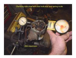
Over time things wear out and with distributors they are assembled with grease and grease can turn into a very hard substance over time and decrease the performance. It is a very good idea to completely disassemble the distributor and clean and wash all the parts with a good cleaner or solvent. Once you have everything cleaned you can check the condition of the parts to either replace them or reuse them.
