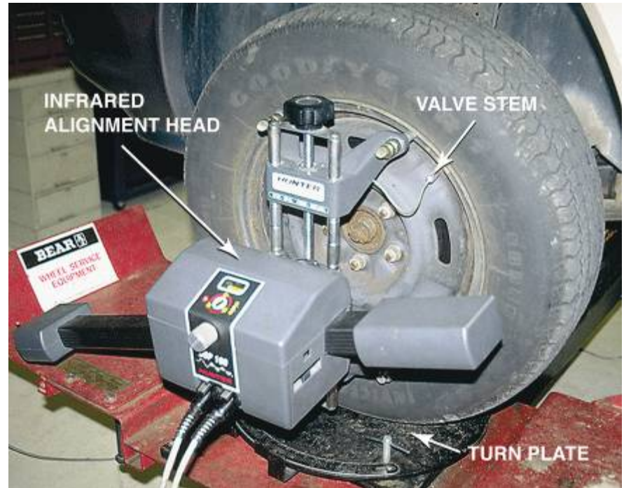
FIGURE 34–11 This wheel sensor has a safety wire that screws to the valve stem to keep the sensor from falling onto the ground if the clamps slip on the wheel lip.
