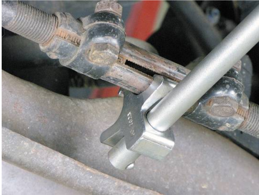
FIGURE 34–39 Special tie rod adjusting tools should be used to rotate the tie rod adjusting sleeves. The tool grips the slot in the sleeve and allows the service technician to rotate the sleeve without squeezing or damaging the sleeve.
