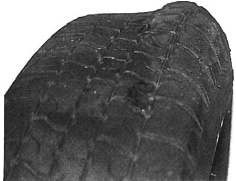
FIGURE 34–6 The bulge in this tire was not noticed until it was removed from the vehicle as part of a routine brake inspection. After replacing this tire, the vehicle stopped pulling and vibrating.
