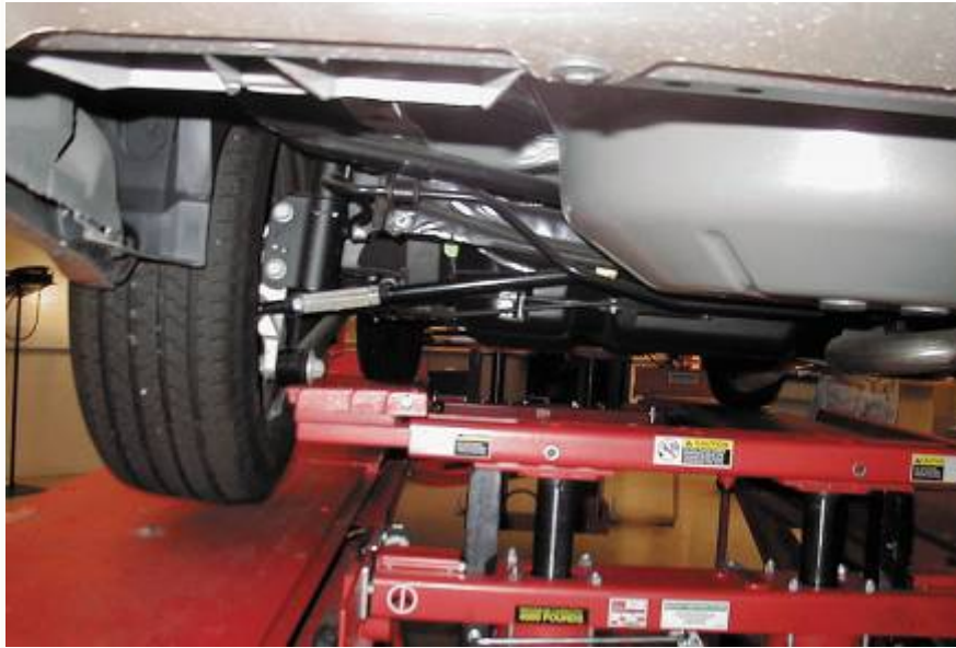
FIGURE 34–10 Using the alignment rack hydraulic jacks, raise the tires off the rack so that they can be rotated as part of the compensating process.
