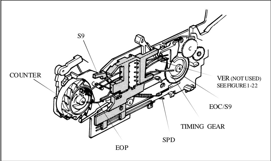
Figure 1-19. Wireform Switchblock and Drive Assembly
