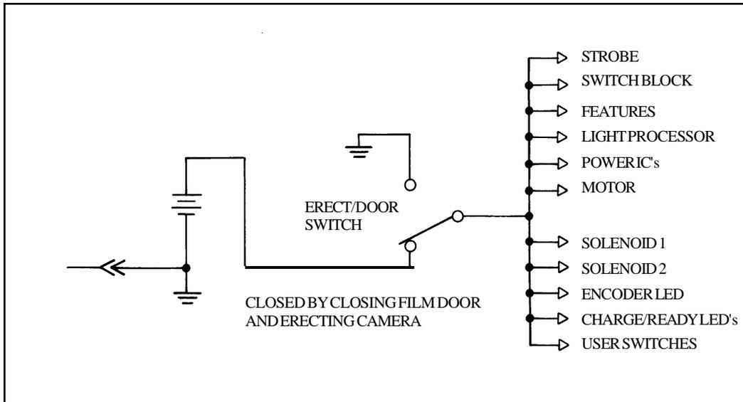
Figure 1-23. Electrical Circuits with Door Closed and Camera Erected
