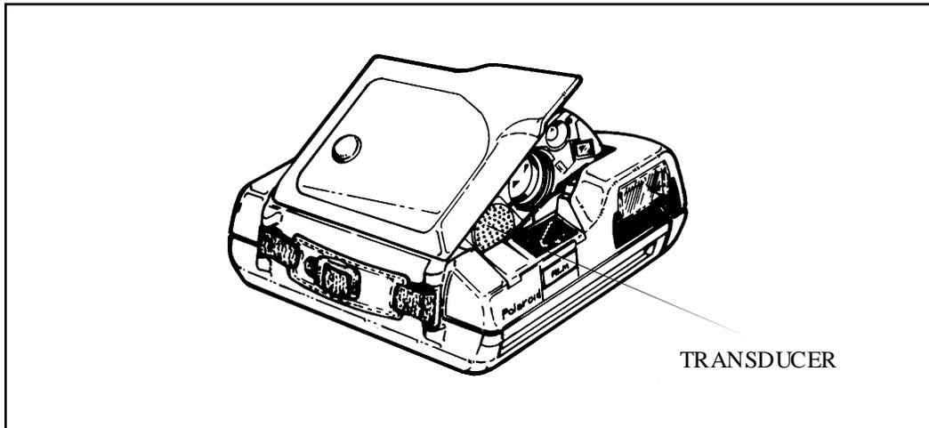
Figure 1-16. ProCam System Transducer
