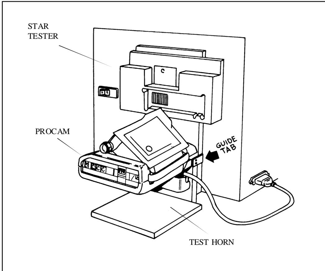
Figure 2-4. Positioning ProCam on Test Horn against Tester.
