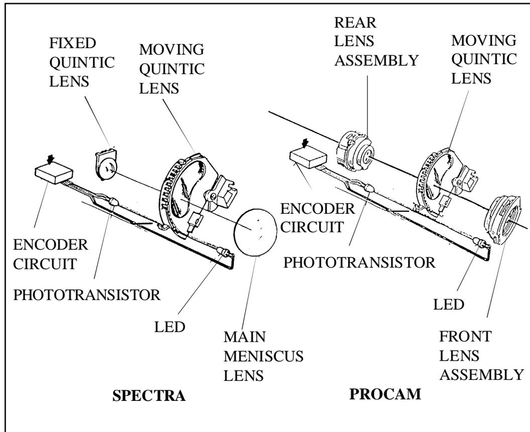
Figure 1-5. Comparison of Spectra and ProCam Quintic Lens Systems
