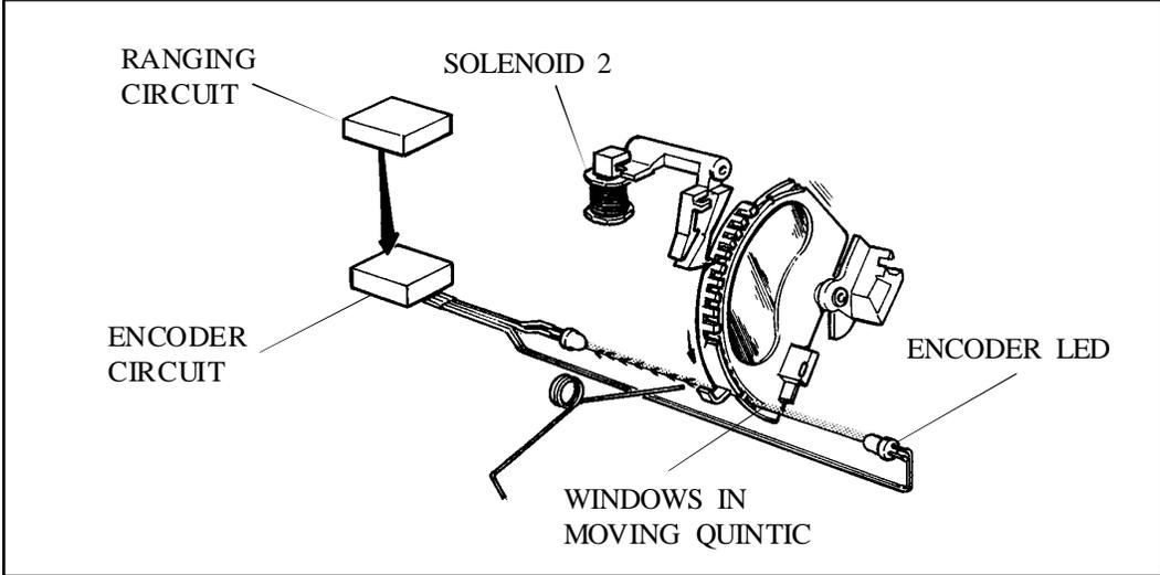
Figure 1-29. Encoder Circuit Reads Light Pulses
