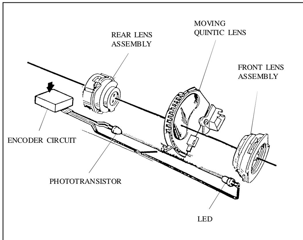
Figure 1-8. Components of ProCam Quintic Lens System
