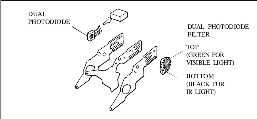
Figure 1-15. Dual Photodiode
