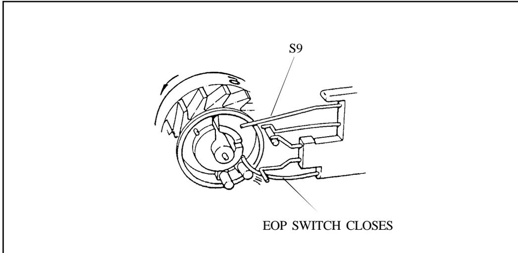
Figure 1-36. Closing the EOP (End Of Pack) Switch
