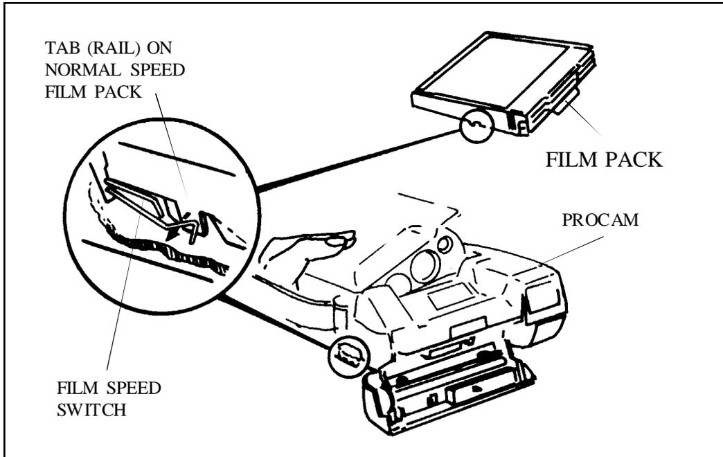
Figure 1-20. Film Speed Wireform Switch
