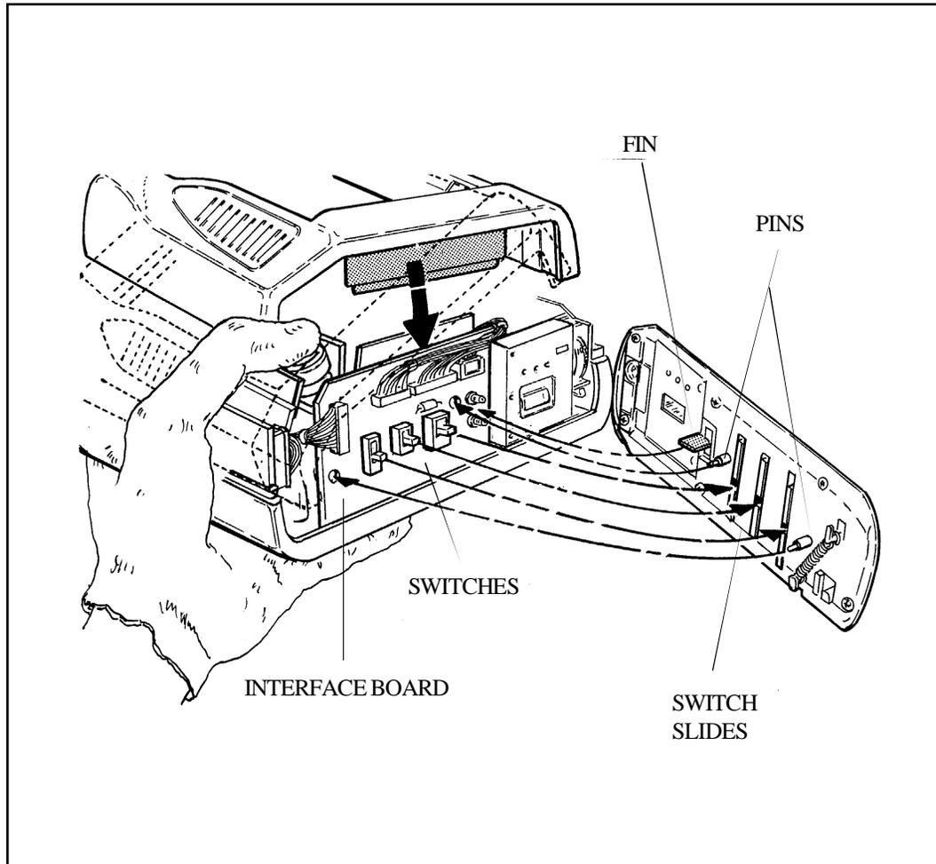
Figure 3-20. Replacing Rear Panel Assembly
