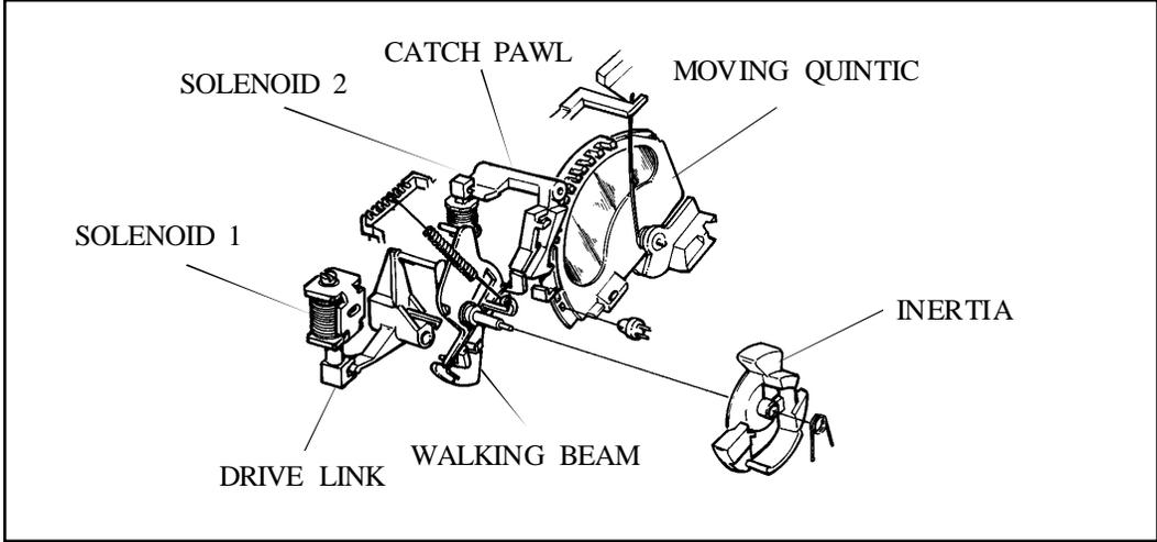
Figure 1-27. Quintic Lens System in Starting Condition
