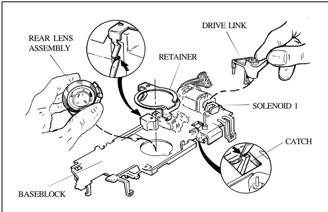
Figure 3-42. Removing Drive Link and Rear Lens Assembly from Baseblock
