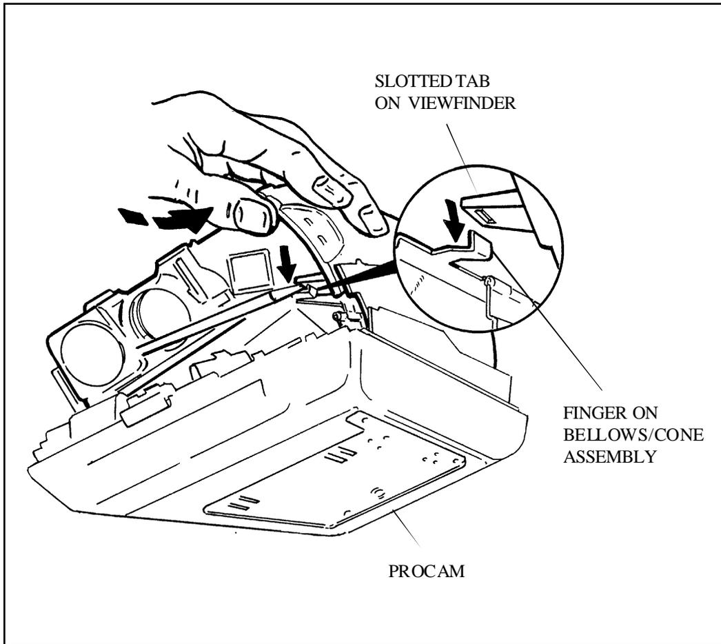
Figure 3-7. Removing Viewfinder Assembly
