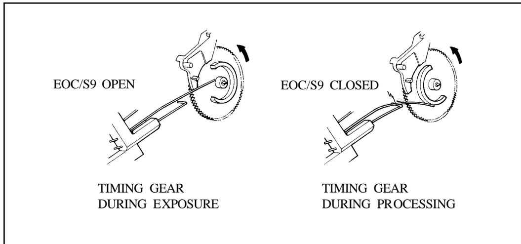
Figure 1-34. EOC/S9 Wireform Switch Closed by Timing Gear Cam
