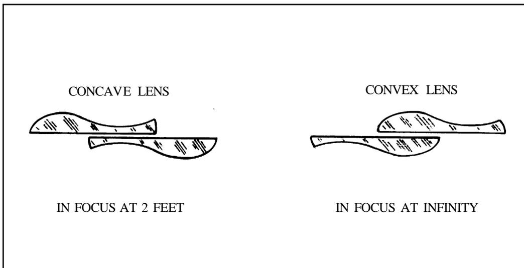
Figure 1-7. Interaction of Aspheric Lenses
