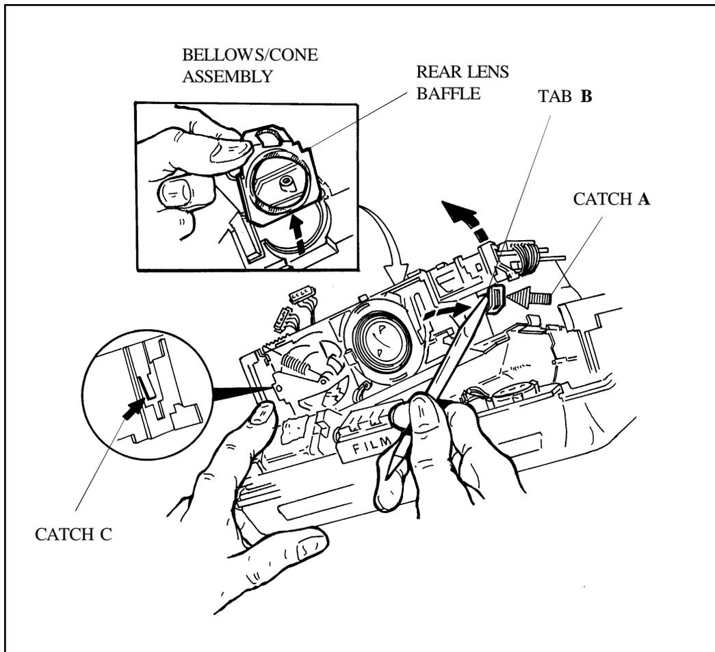
Figure 3-14. Removing Shutter Assembly from Bellows/Cone Assembly
