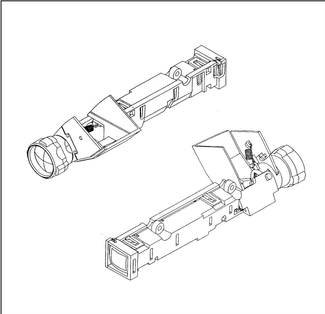
Figure 1-3. ProCam Camera Viewfinder Assembly
