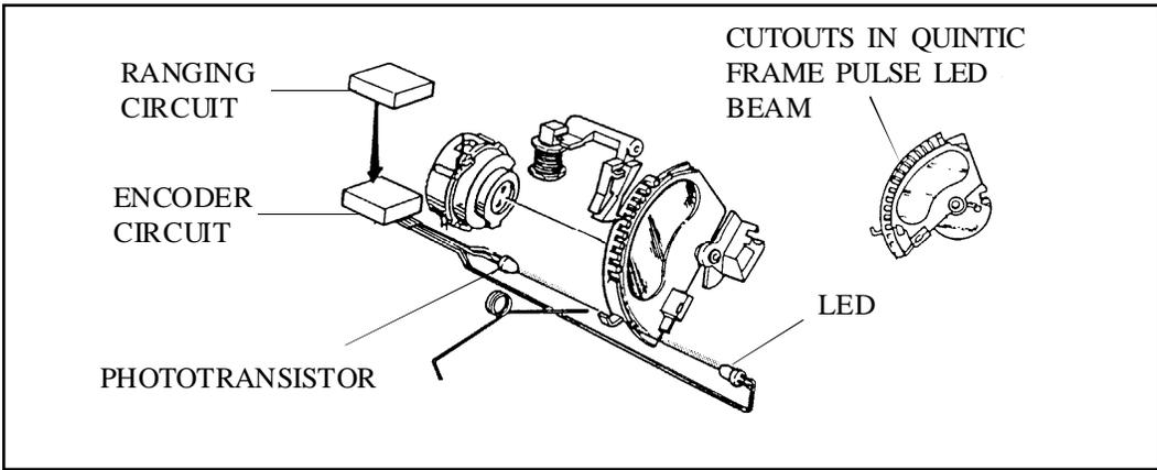
Figure 1-11. Encoder Circuit Detects LED Light Pulses
