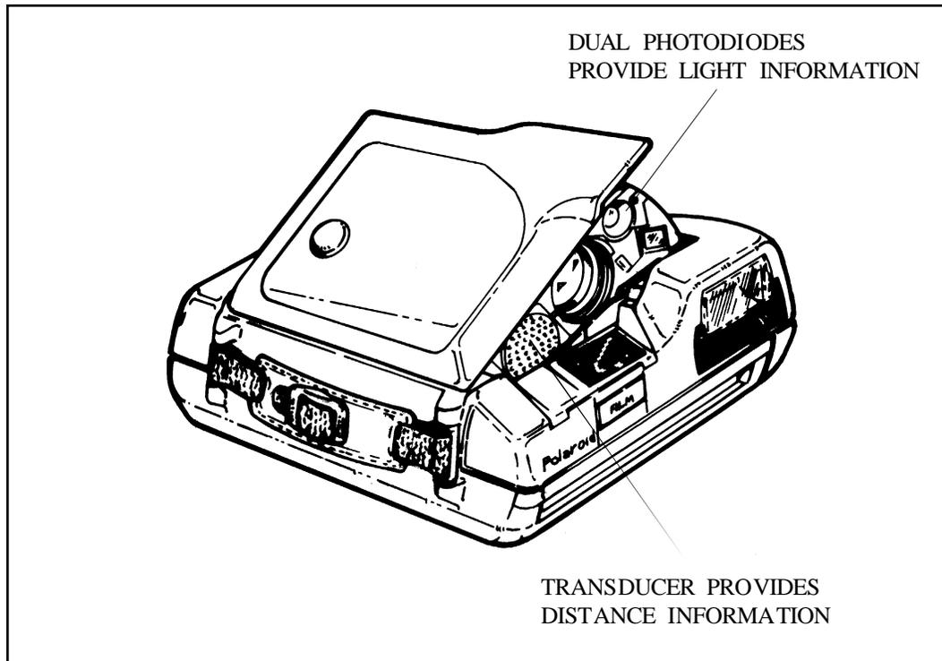
Figure 1-13. Hybrid Light and Distance Measurements
