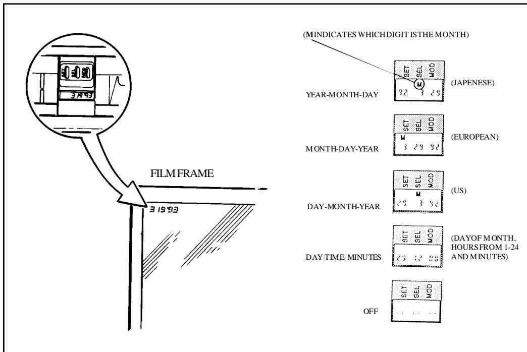
Figure 1-18. User-selectable Date and Time Imprints on ProCam Pictures
