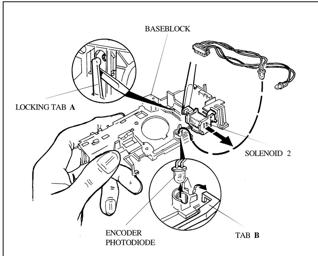
Figure 3-44. Removing Solenoid 2 and Photodiode from Baseblock
