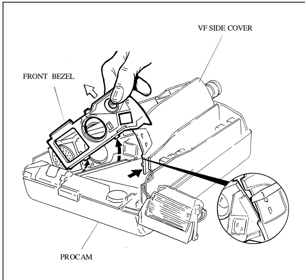
Figure 3-6. Removing Front Bezel
