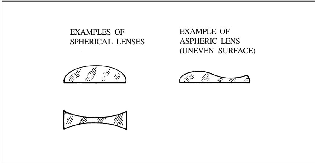
Figure 1-6. Comparison of Spherical and Aspherical lenses
