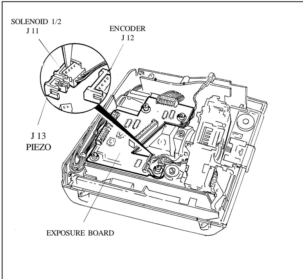
Figure 3-12. Encoder, Piezo and Solenoid 1/2 Connectors on Exposure Board
