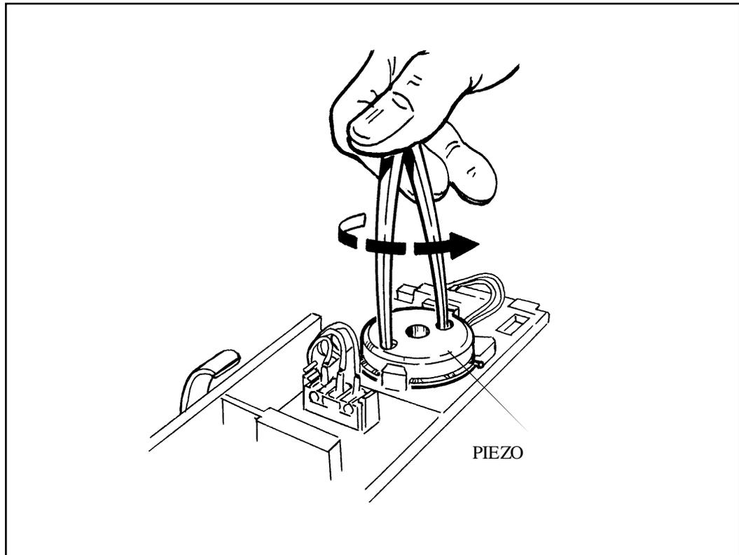
Figure 3-34. Removing Piezo from Mainframe
