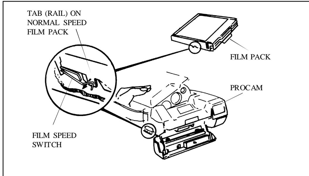
Figure 1-17. Film Speed Switch
