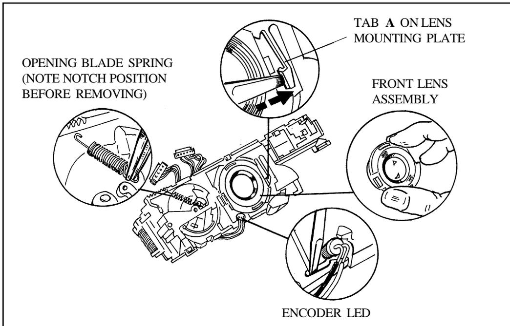
Figure 3-37. Removing Front Lens, Encoder LED and Opening Blade Spring
