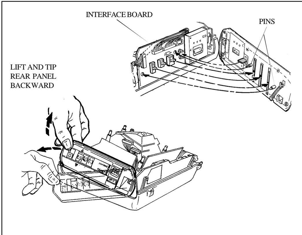
Figure 3-19. Removing Rear Panel Assembly
