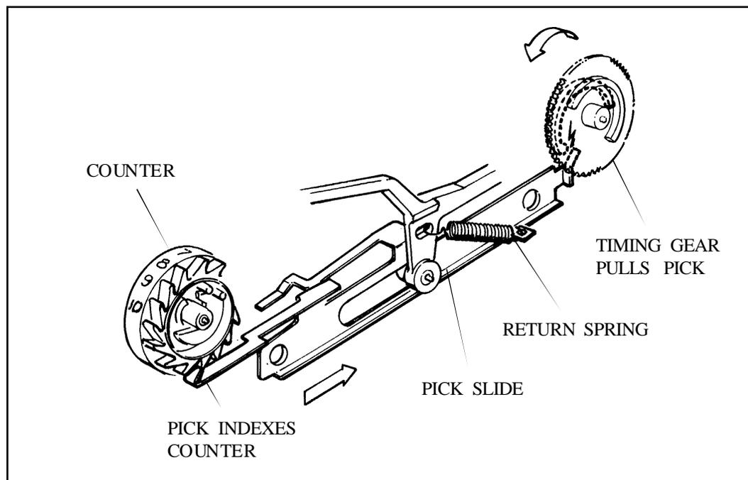
Figure 1-25. Pick Slide Ejecting Dark Slide and Indexing Counter
