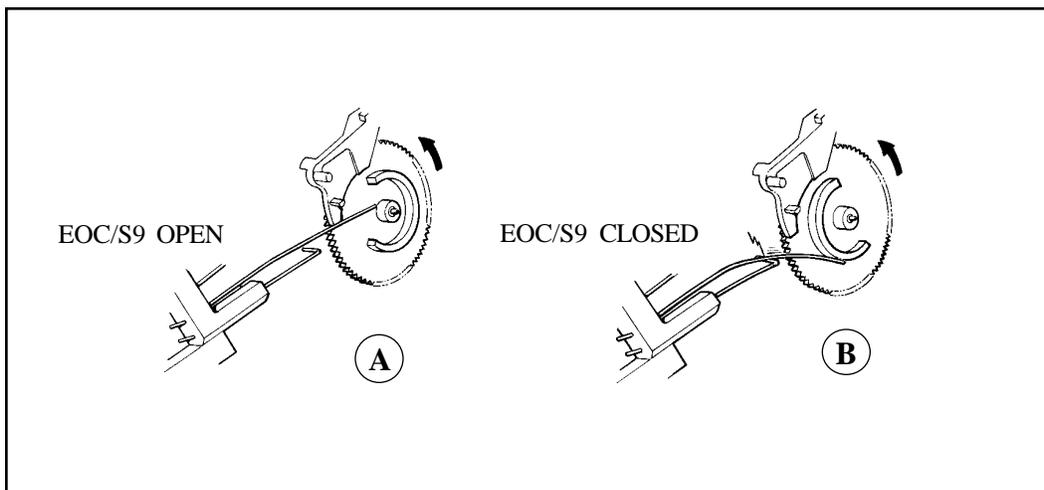
Figure 1-24. Timing Gear Closing EOC/S9
