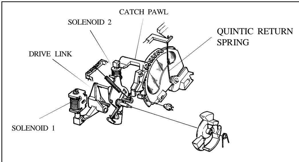
Figure 1-33. Shutter Components at End of Exposure Cycle
