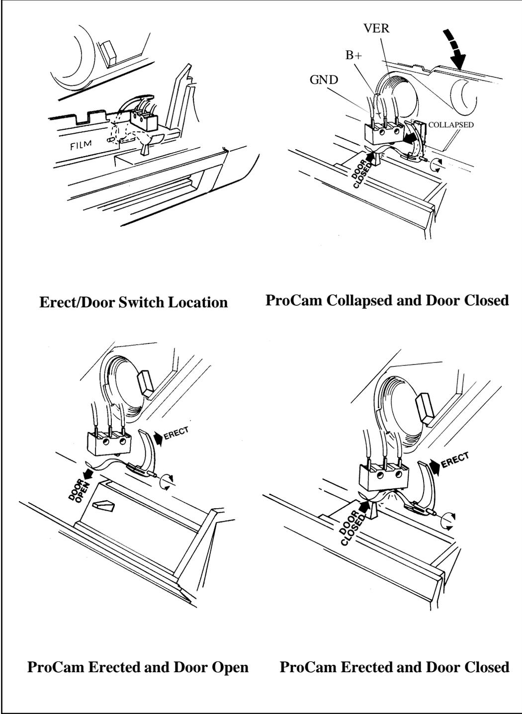
Figure 1-22. Door/Erect Switch Closure
