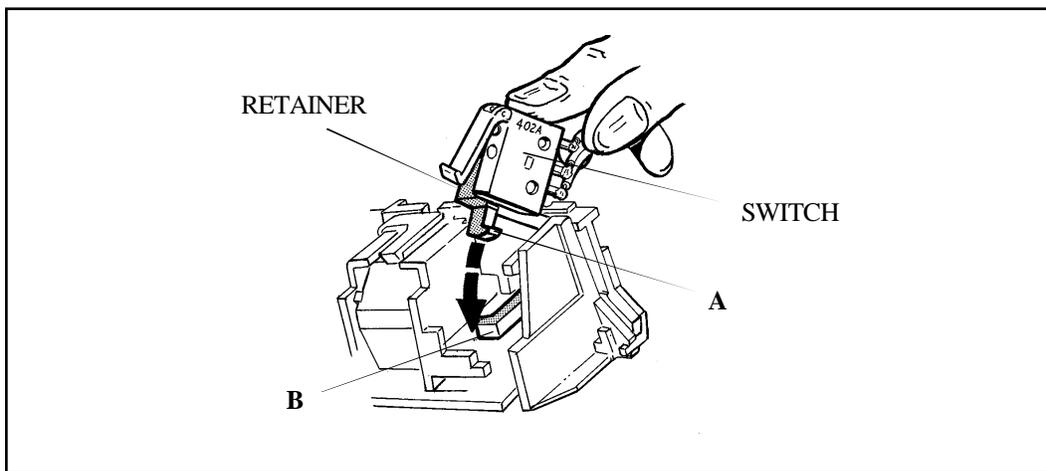
Figure 3-10. Replacing Close-Up Lens Switch/Retainer in the Lens Mounting Plate
