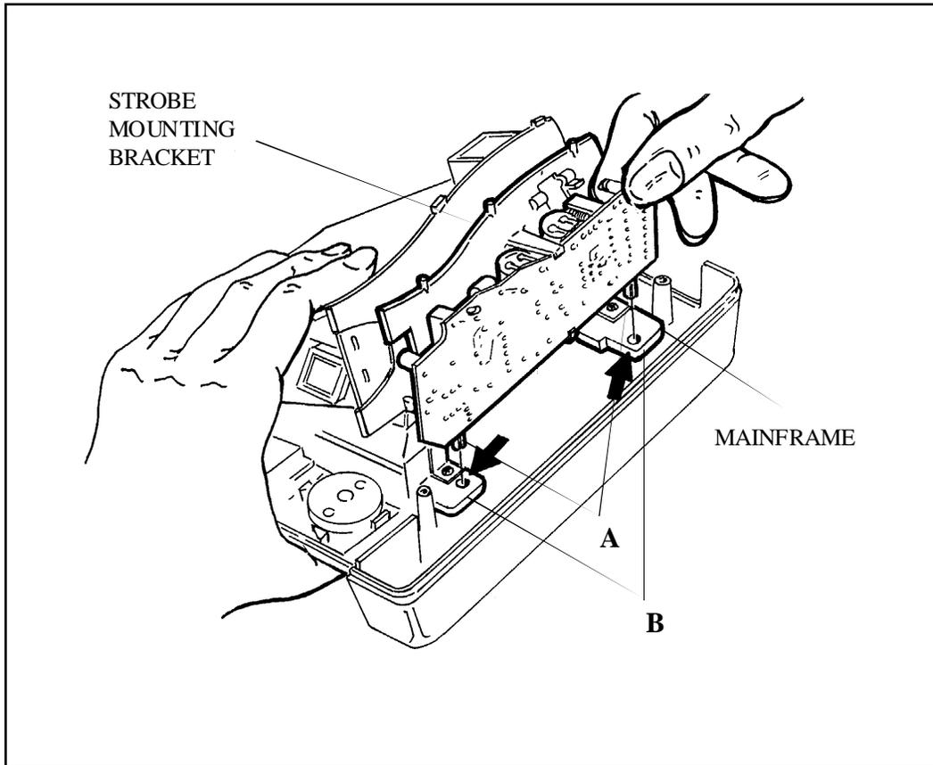
Figure 3-24. Seating Strobe Mounting Bracket
