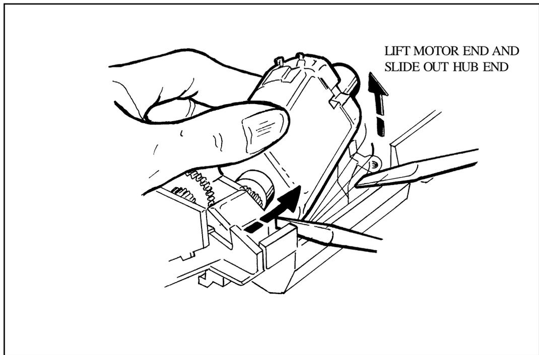
Figure 3-36. Removing Motor from Mainframe
