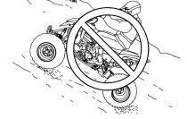
Never open the throttle suddenly. The ATV could flip over backwards. Never go over the top of any hill at high speed. An obstacle, a sharp drop, or another vehicle or person could be on the other side of the hill.
