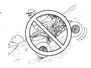
If you begin rolling backwards: Keep weight uphill. Never apply engine power. Never apply the rear brake while rolling backwards. Apply the front brake slowly. When fully stopped, apply rear brake as well, and then lock the parking brake. Dismount on uphill side, or to either side if pointed straight uphill. Turn the ATV around and remount, following the procedure described in the Owner's Manual. See page 102.
