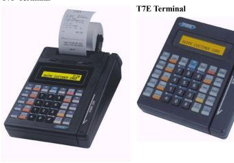
The T7P has a built in printer. Both the T7E and T7P have no RS-232 port to plug in a check reader. An additional piece of hardware (called the FIP 11) can be purchased for the T7P that allows a check reader to be plugged in.
