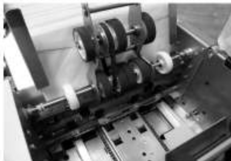
Figure 3: Outer lower tyres removed from the pre-feed assembly
