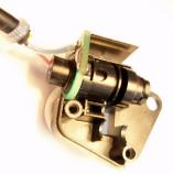
3. Place the Push Bar (52) together with the Filter Holder (58) as shown. Note the orientation of the parts with each other.
