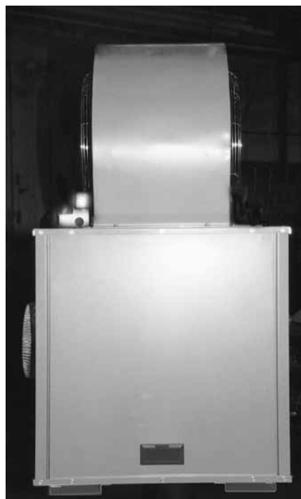
Heat Exchanger/ Combustion Chamber Outer Access Door
