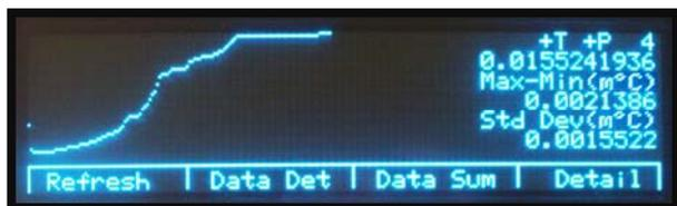
The model 6622T thermometry bridge can be used in either a **fixed or dynamic reversal rate** mode of operation. In fixed reversal rate mode, **automatic current polarity reversal is user programmable** from 4 seconds to 27 minutes with two measurements per reversal. Dynamic reversal rate mode is only available in computerized measurements, where the bridge software **optimizes the polarity reversal rate** in real time. In temperature applications, this feature makes it easy to **track a**
