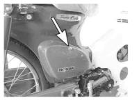
2 . From the main harness, remove the coupler connected to a genuine ECU. And unfasten the screw holding a battery cover.
