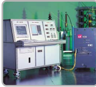
Characteristics Test / VCB Characteristics Test
