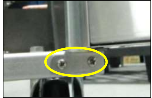
Remove the two mounting screws of the door hinge bracket
