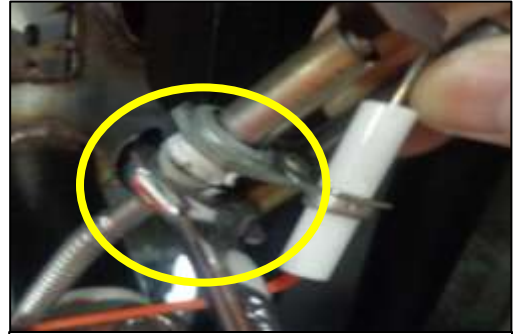
Disconnect the pilot tube from the FDS
