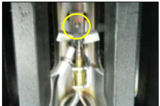
Remove the mounting screw of the FDS
