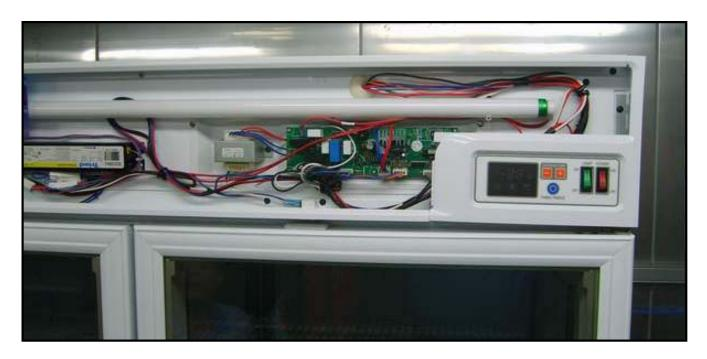
D. Replace parts as needed (Display board, Power switch, Lamp switch)
