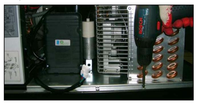
D. Slide out the Condensing Unit to replace the fan motor and the compressor.
