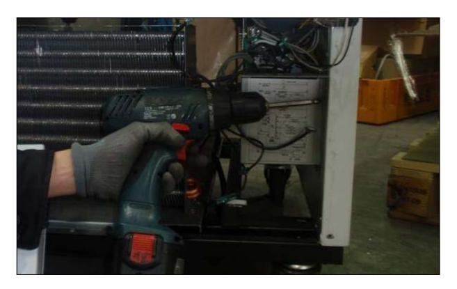
D. Replace the Main PCB, Transformer, and Magnetic contactor.
