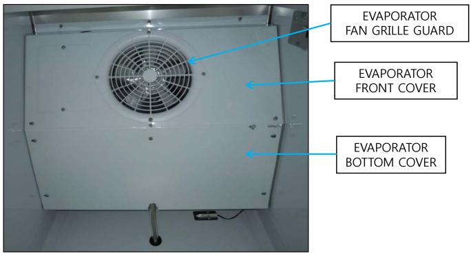
► EVAPORATOR, FAN MOTOR, DEFROST HEATER, SENSORS(TGIM-23\*)
