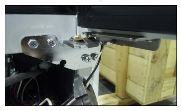
C. Remove the Sign Frame(Left, Right) by unscrewing the four screws of each side.
