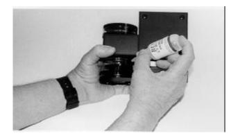
C. Wet flow cell by connecting a pump flowing at 1000 to 2000 cc/min. for Model M-5 and 5 LPM for Model M-30. Initiate soap film up center tube by rapidly pressing button down and releasing. Repeat this procedure until bubble doesn't break. The tube is now wet and tests at any range may be conducted. One minute warm up time is all that is required of the mini-Buck.
