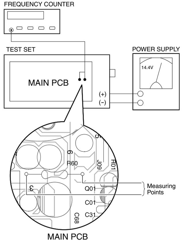
2. Measure the secondary toroidal coil, if the standard frequency value of 22.87 kHz ± 50 Hz is not attained, measure the R60 terminal, then adjust the SV01 so that the R60 terminal becomes 22.87 kHz ± 50Hz.
