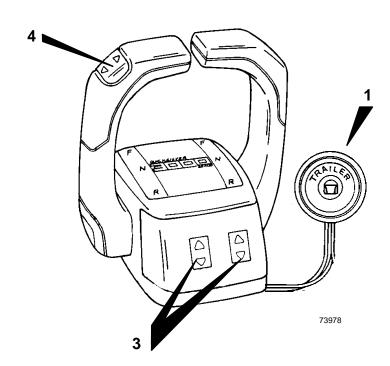
POWER TRIM OPERATION - DUAL ENGINE CONSOLE MOUNT REMOTE CONTROL (TWO BUTTON AND THREE BUTTON VERSIONS)
