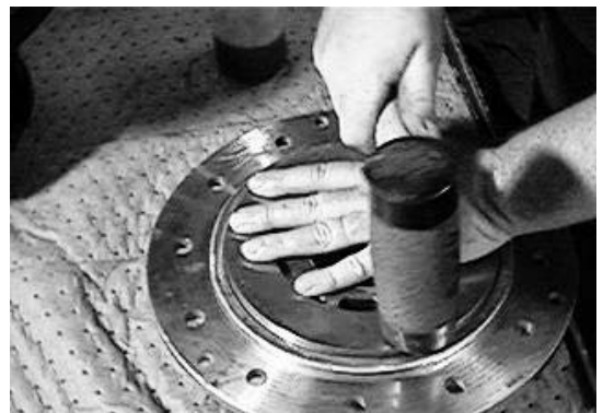
Use rubber hammer to install clutch piston.
