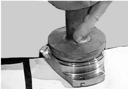
Use proper driver to install inner lip seal.
