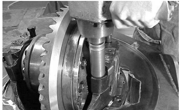
Loosen (4) cap bolts.
