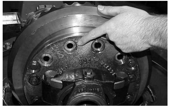
Rotate the ring gear until the empty holes align with the pinion.
