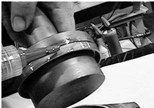
Apply Loctite #620 to outer lip seal.
