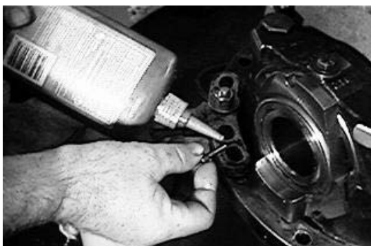
Apply Loctite #262 to capscrews.
