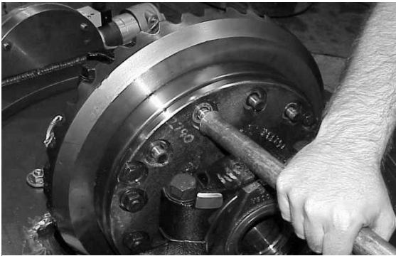
Carefully remove the (4) bolts with a brass driver.
