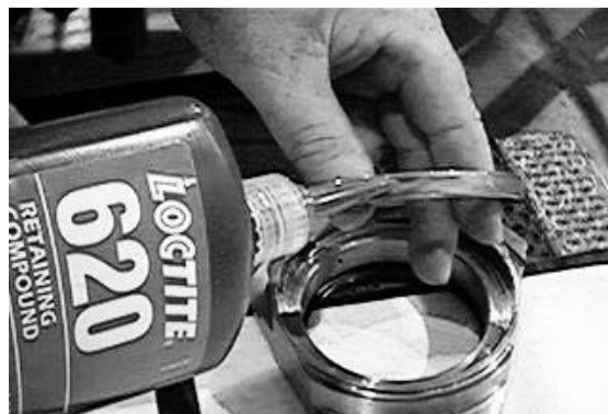
Lightly apply Loctite #620 to inner lip seal.
