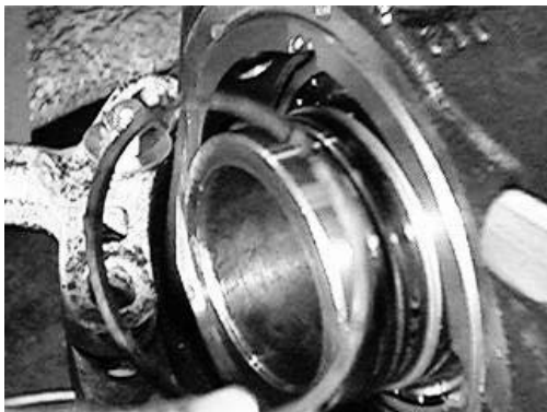
Install piston rings.
