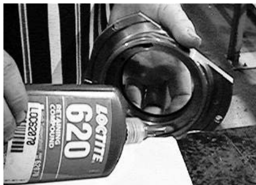
Apply Loctite #620 to seal retainer.
