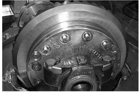
Remove the (4) nuts.
