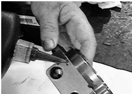
Apply Loctite #262 to seal retainer.
