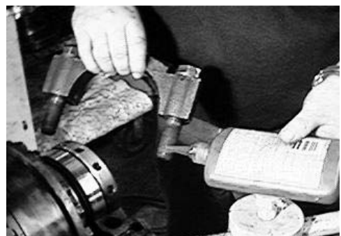
Apply Loctite #262 to capscrews.
