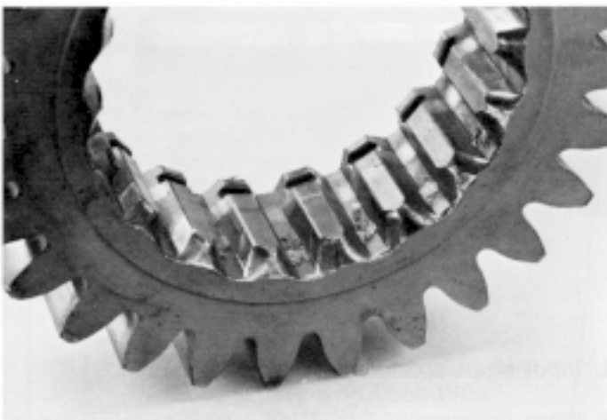
Snubbed clutching teeth
