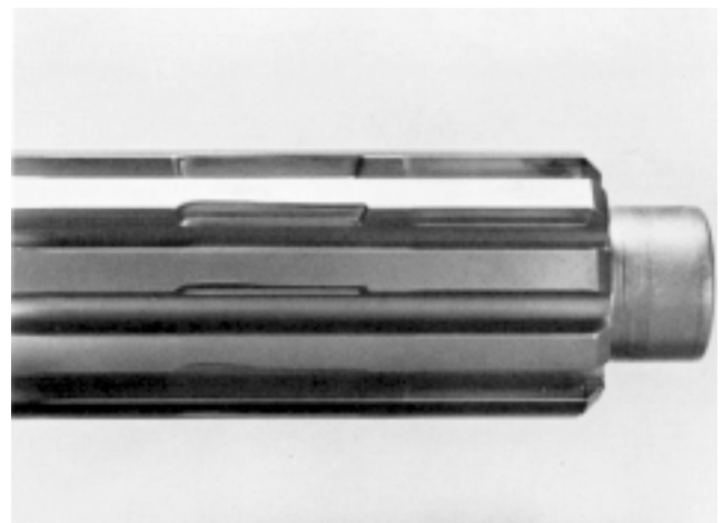
Input spline wear
