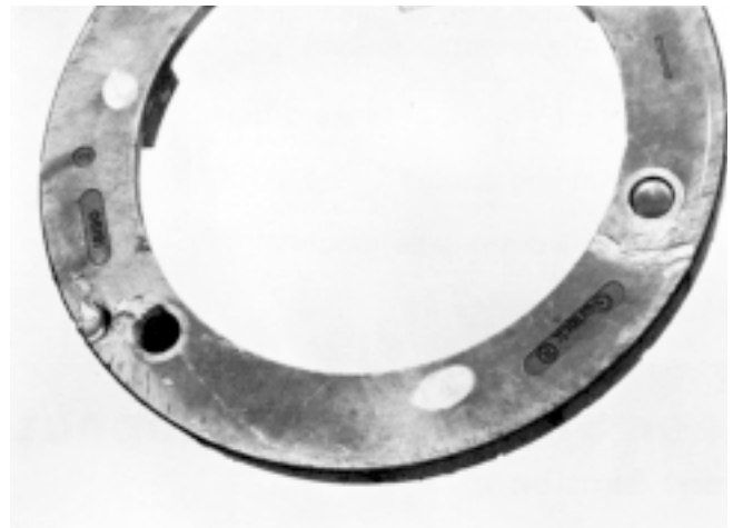
Broken synchronizer pins
