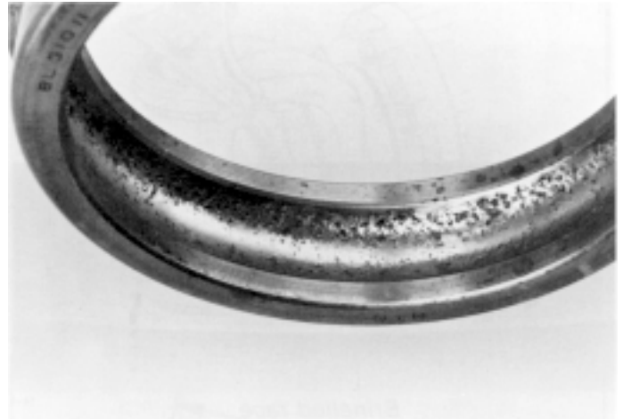
Burnt and spalled bearing 13-3
