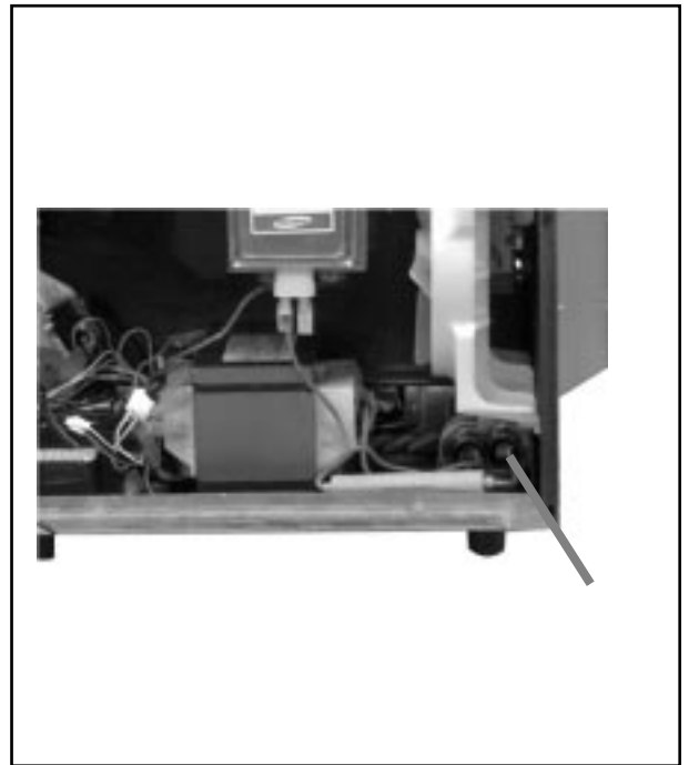
Fig. 1-1. Discharging the High Voltage Capacitor
