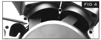
Caution: When grinding and filing cylinder, you must maintain a smooth finish, without making sharp corners.
