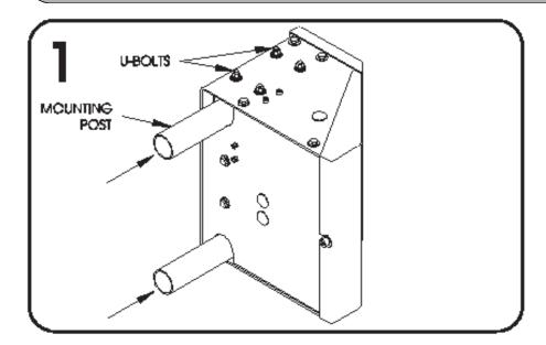
O For post mount installation, install the posts onto the the gate operator. The posts are first insterted up into the bottom the gate operator. The posts are secured by tightening u-bolt nuts from the outside.
