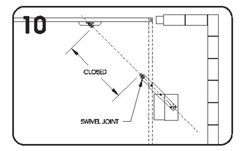
to be cut to a length appropriate for the specific location chosen for the gate operator. First put the gate into the close position and point the primary arm toward the gate bracket. Be sure the the swivel joints are also pointing toward each other. Measure the distance between the two swivel joints.
