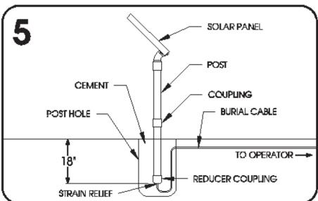
O If the gate operator is solar powered, no power will need to be run into the machine. The ends of the wires are provided with connectors which can simply be plugged in. Turn the panel so that it will get maximum sunlight during the day. If necessary the panel may be mounted away from the gate operator to get it out of the shade and into more consistent sunlight.
