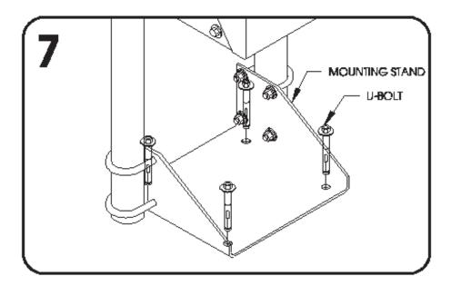
intallation, first place the operator with concrete mounting stand at it's desired location on the concrete surface. It is necessary to first mark through the holes onto the concrete, then remove the operator to drill the holes with a 3/8" masonry bit. The operator may then be set back in place. Insert the 3/8" sleave anchors into the holes and tighten.
