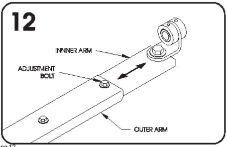
O If the two measurements are not the same. It will be necessary to adjust the length of the primary arm by loosening the two bolts on the primary arm. Repeat the above measurements until the two measurements are equal. Once equal, securely tighten the two bolts on the primary arm.
