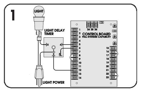
O If it is desired that the driveway illuminate when the gate is activated, a light delay timer may be installed. The light delay timer will switch power on to the light for two minutes, then shut power back off. The timer relay is capable of switching up to 10 Amps which will handle most flood or spot lights available. A general hook-up diagram for the light and timer is shown at left.
