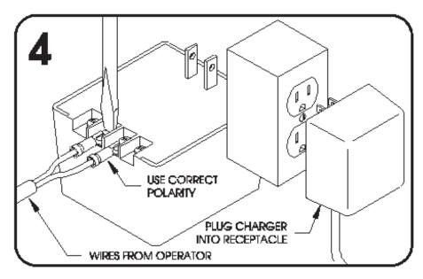
O Connect the other end of the burial cable from the operator to the float charger. Be sure to match the positive and negative terminals of the charger to the positive and negative terminals of the battery. Once the connections are made, plug the charger into a 115 Volt outlet. If possible, it is desirable to locate the charger out of the weather. Let the charger charge the battery for a couple of hours before putting into operation.
