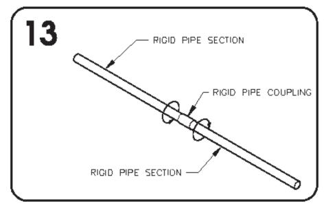
in two peices and must be assembled. Connect the two pipe arm together with the pipe coupling and securely tighten them.
