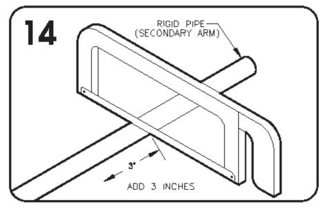
O Use the measurement from adjusting the primary arm to determine the length of the secondary pipe arm. Take the previously determined measurement and add 3 inches. This allows for the extra pipe that is necessary to protrude into the swivel joint. Cut the arm with hack saw.
