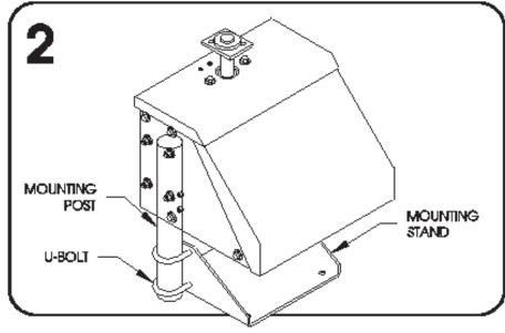
O For optional concrete pad mount installation, short posts are installed onto the gate opener and secured by tightening the u-bolt nuts from the outside. The concrete pad mounting plate is then installed onto the bottom of the posts.
