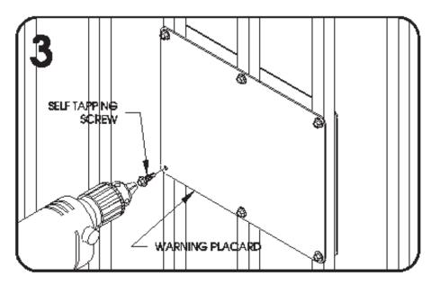
O See the illustration at left for an example of how the warning placards may be fastened to the gate with the use of self tapping sheet metal screws.
