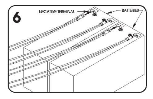
O Similarly to the battery back-up, the solar operator comes with the battery wires disconnected. For both batteries, connect the black wires to the negative terminals and the red wires to the positive terminals. The wires have been labeled to make these connections easier to do.
