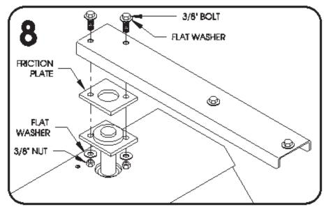
• Attach the primary arm onto the end of the operator shaft as shown. It may be convenient to not completly tighten the bolts securing the arm at this point.
