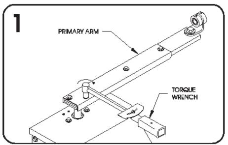
O The primary arm is designed to clamp onto the output shaft in such a way that the arm will slip on the shaft in the event that an obstruction exists in the path of the gate. The bolts for securing the primary arm should be tightened to a torque that will cause the gate to push with minumum force. Tighten both bolts with equal torque, then push on the end of the gate to determine the amount of force necessary to cuase the arm to slip.
