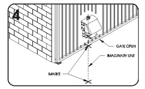
mate location so that the center of the shaft is located along the line that was previously drawn. Allow some clearance for the gate so the gate will not run into the gate opener during operation.
