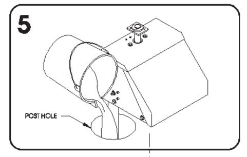
O When the gate operator location has been determined, make two post holes at the location of the posts. Place the operator with posts so that the posts protrude down into the post holes. Set the operator at the desired hieght from the ground. Secure the operator from movement and pour concrete into the holes. Allow adequate time for the concrete to harden.
