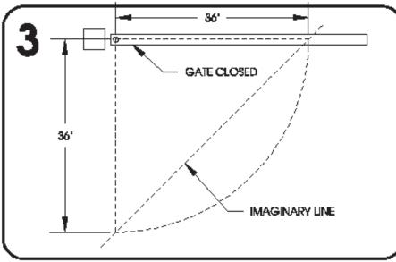
O Determine the location where the operator is to be installed permenently. First close the gate and make a mark on the ground below the gate at 36" from the hinge. When done, open the gate and again make a mark on the ground at 36" from the hinge. A line may then be drawn though the two marks on the ground. The operator will then be placed so the the shaft lies on the line.
