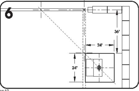
O If there is no existing concrete pad, and the gate operator will be concrete pad mounted, use the illustration at left as a guide for locating and sizing the concrete pad. A 2ft x 2ft pad is recomended for installation, with at least 6" of depth into the ground.
