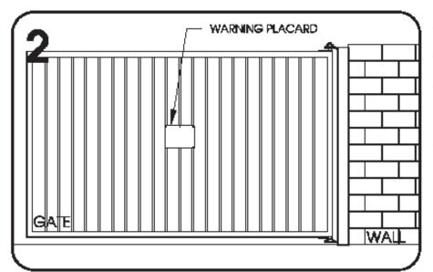
O The gate operator is provided with two safety warning placards. The placards are to be installed on each side of the gate where they are plainly visible. The placards may be mounted using sheet metal screws through the six holes provided on each placard.
