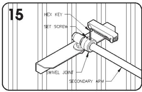
O When the pipe arm has been cut, it may be attached to the gate operator and gate bracket. Insert the pipe into both the swivel joint on the primary arm, and the swivel joint on the gate bracket. Secure the pipe arm to both swivel joints by tightening the set screws on the swivel joints.
