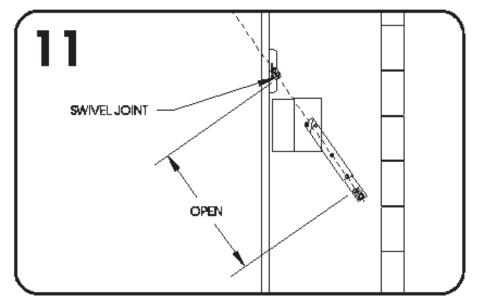
O Put the gate into the open position and point the primary arm away from the gate bracket. Again be sure that the swivel joints are pointing toward each other. Measure the distance between the gate brackets. Compare the measurement to the previous measurement from the close position. The measurements should be the same.
