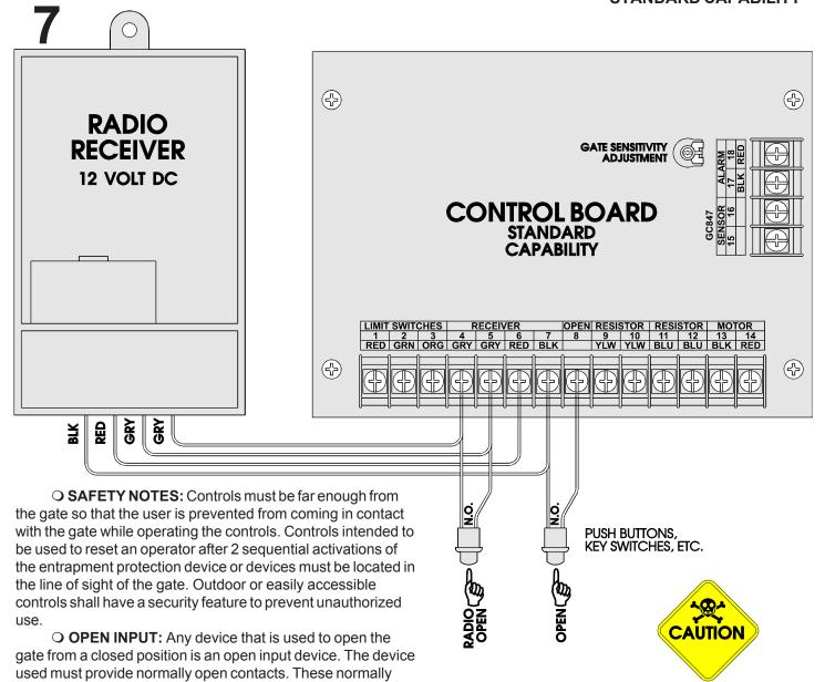
TO AVOID POSSIBLE INJURY OR DAMAGE TO EQUIPMENT DO NOT MAKE ELECTRICAL CONNECTIONS WHILE POWER IS ON
