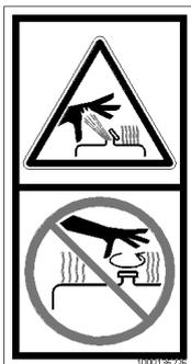
Fig. 19: Hydraulic oil tank under pressure
