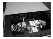
6. Loosen center bulb bracket retaining screws, if needed, for bulb clearance.
