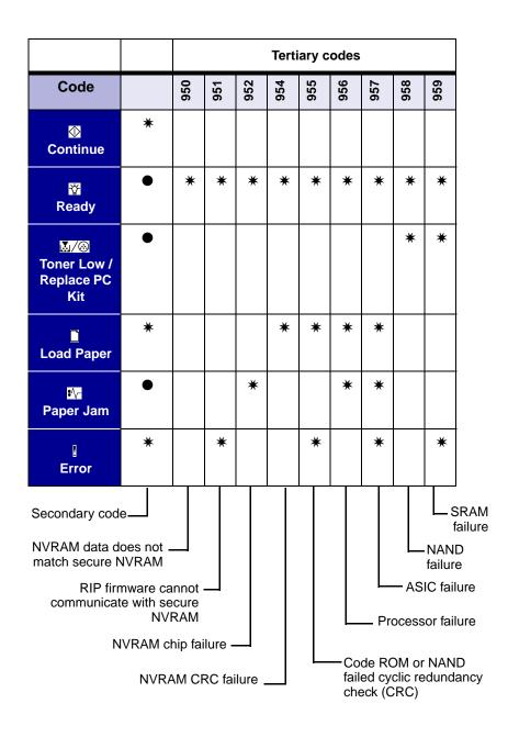
**Note:** NVRAM is on the operator panel printed circuit board (PCB) while secure NVRAM is on the controller PCB. Check margin alignments after replacing the operator panel assembly. See **"Printhead service check" on page 2-61** for more information. If margin errors are unacceptable, corrections can only be made through software. Contact the next level of support or Lexmark at 1-800-539-6275.
