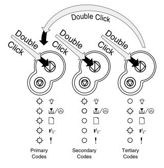
**Note:** All lights flashing simultaneously, as a result of sending data to the printer, may indicate a code problem. Call the next level of support.
