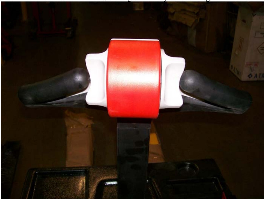
This is the driver side of the tiller, looking at the belly switch. Fig 4
