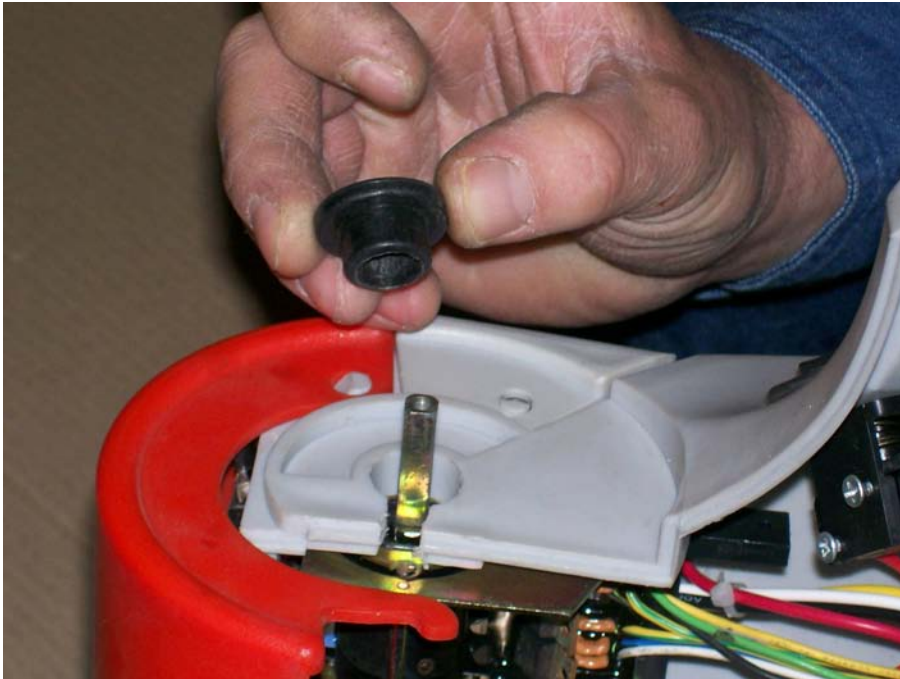
Install bushings. Fig22
