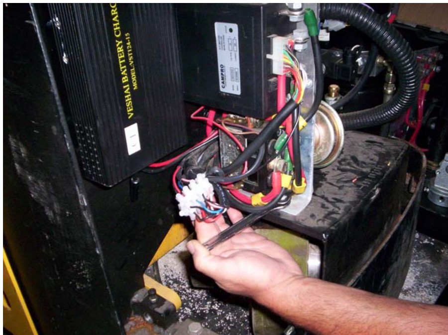
Remove the Molex connector from the motor controller.
