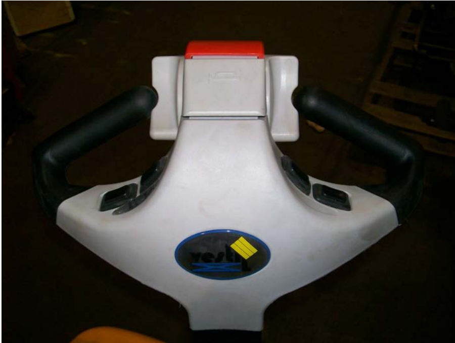
This is the driver side of the tiller, looking at the belly switch. Fig 4
