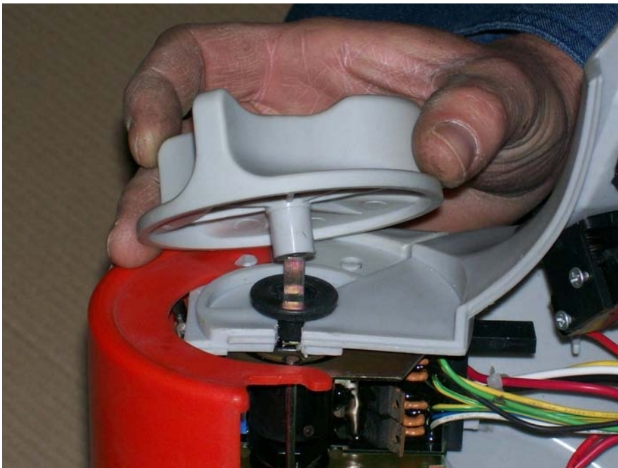
Put throttle thumb wheels back on. Fig23
