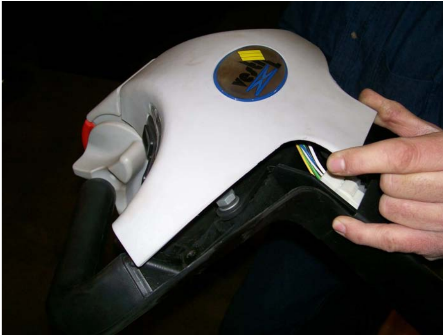
Carefully pull the belly switch back off of the tiller while tipping the front up. Fig 7
