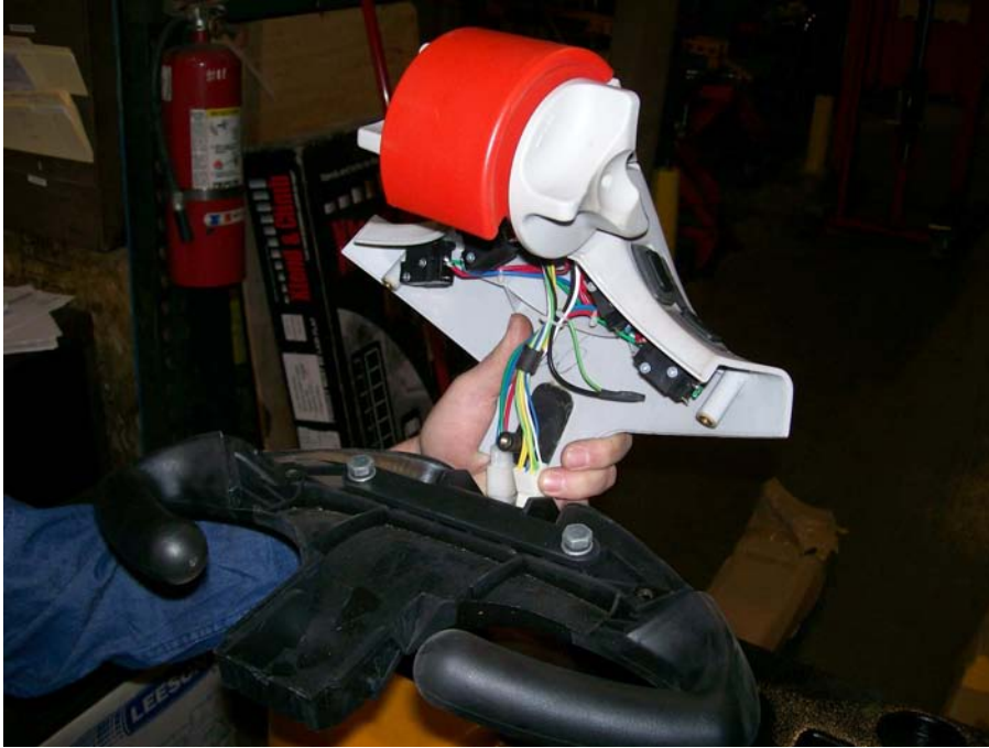
Unplug the two connectors from the tiller throttle assembly. Fig9
