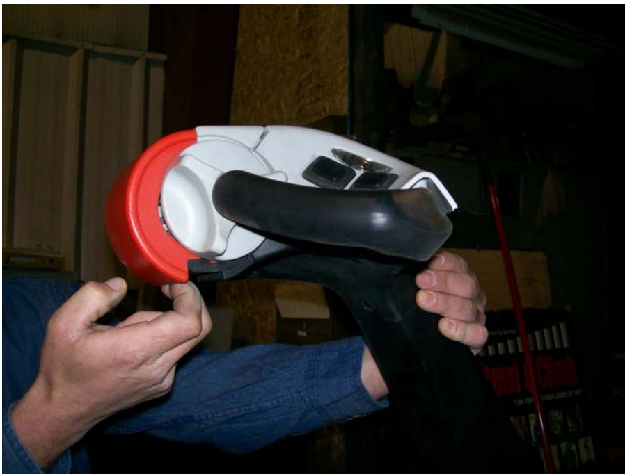
Carefully pull the belly switch back off of the tiller while tipping the front up. Fig 7
