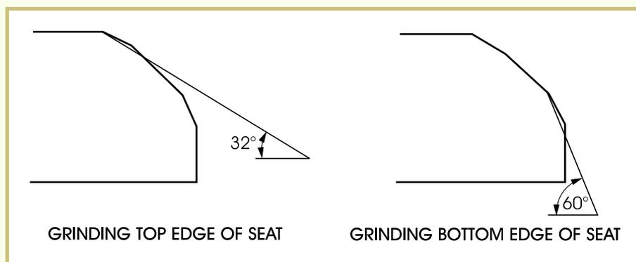
When the seat is narrowed to its proper width, the seat should be finished by cutting it lightly with the 45-degree cutter. This removes any tiny burrs left from narrowing the seat. However, should you narrow the seat by grinding away its top or its bottom? You can decide based on where the valve face makes contact with its seat. (It should be
