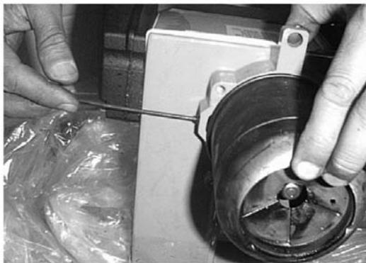
Use 3 mm Allen key to remove flame tube loosening set screws on both sides
