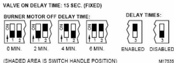
Fig. 8. Switch setting for burner-Off delay times.
