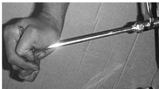
Proceed with reverse process to reinstall the burner after changing the old nozzle with a new 0.5 X 800 AS nozzle
