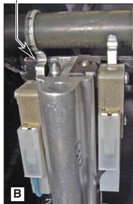
Radius of Tower 4 Microswitch Blade activated by Apex of Activation Plate.
