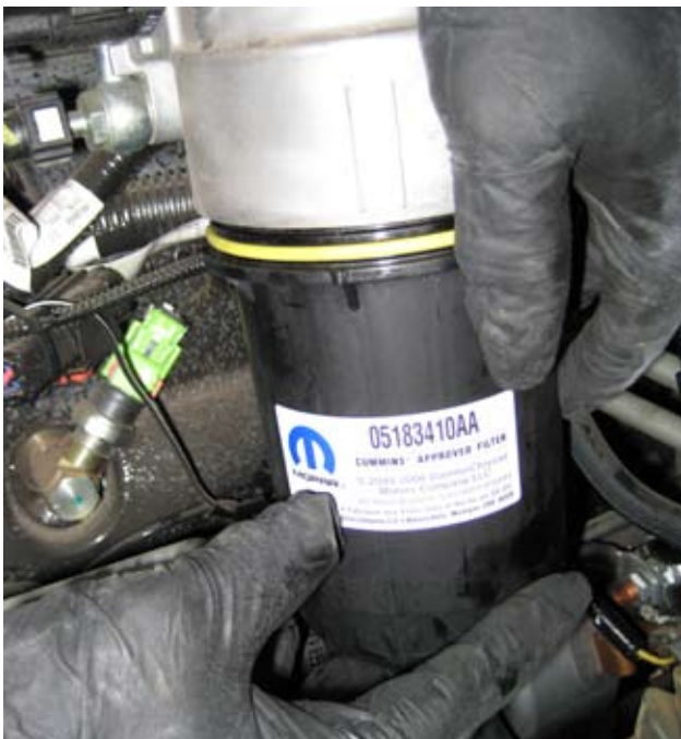
With one hand above and one hand below you can get to the fuel filter from above.
