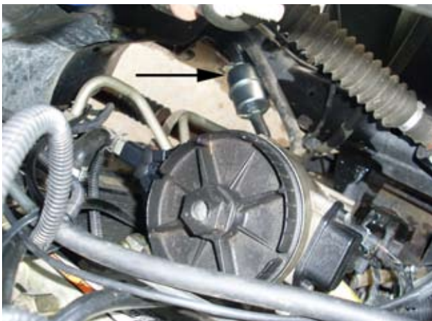
The installed orientation of the new fuel filter.
