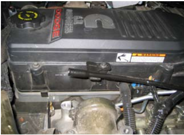
Relocate the oil dipstick tube to the valve cover.
