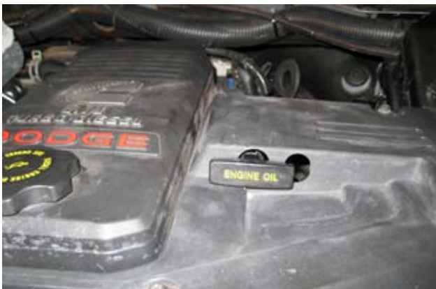
Modified "bat wing" with new dipstick location.
