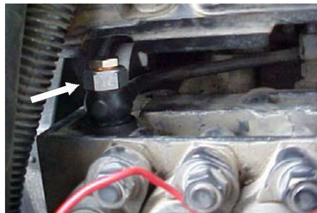
The Bosch P7100 over-flow valve.
