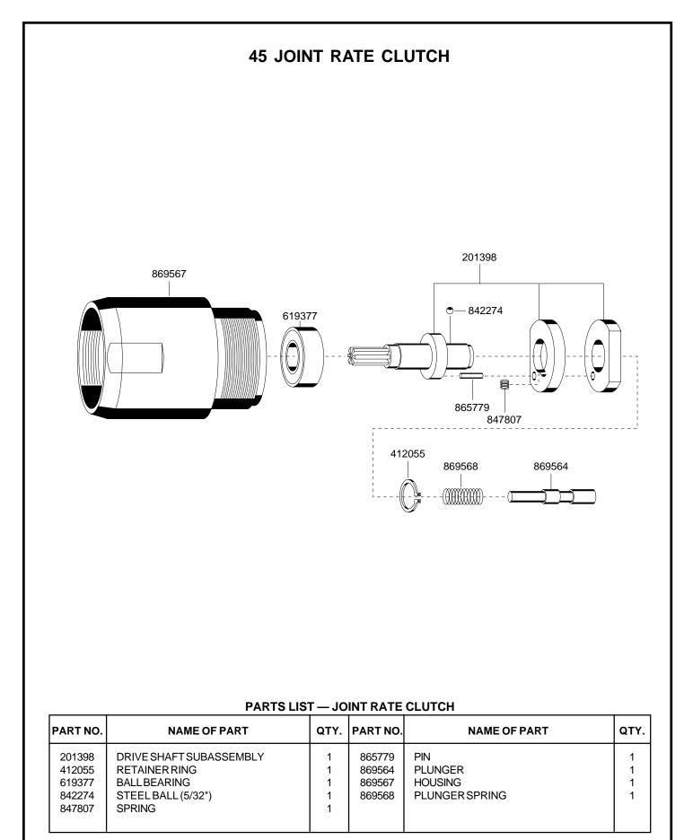
The complete clutch with housing can be purchased as a subassembly using Part No. 861019.
