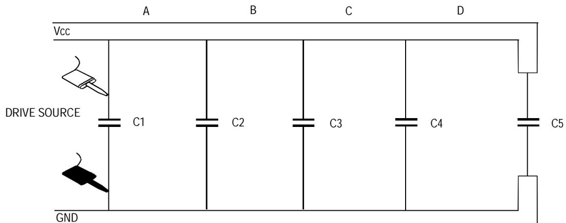
Figure 4-9 Isolation of Open Circuit Decoupling Capacitor
